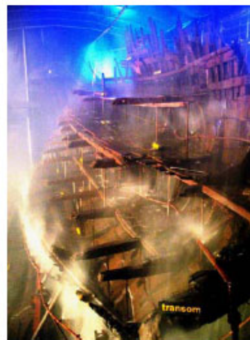
Figure 1. The starboard side of the Mary Rose (about 1/3 of the hull, ~280 tons oak timbers) is since 1994 being sprayed with an aqueous solution of PEG 200.
