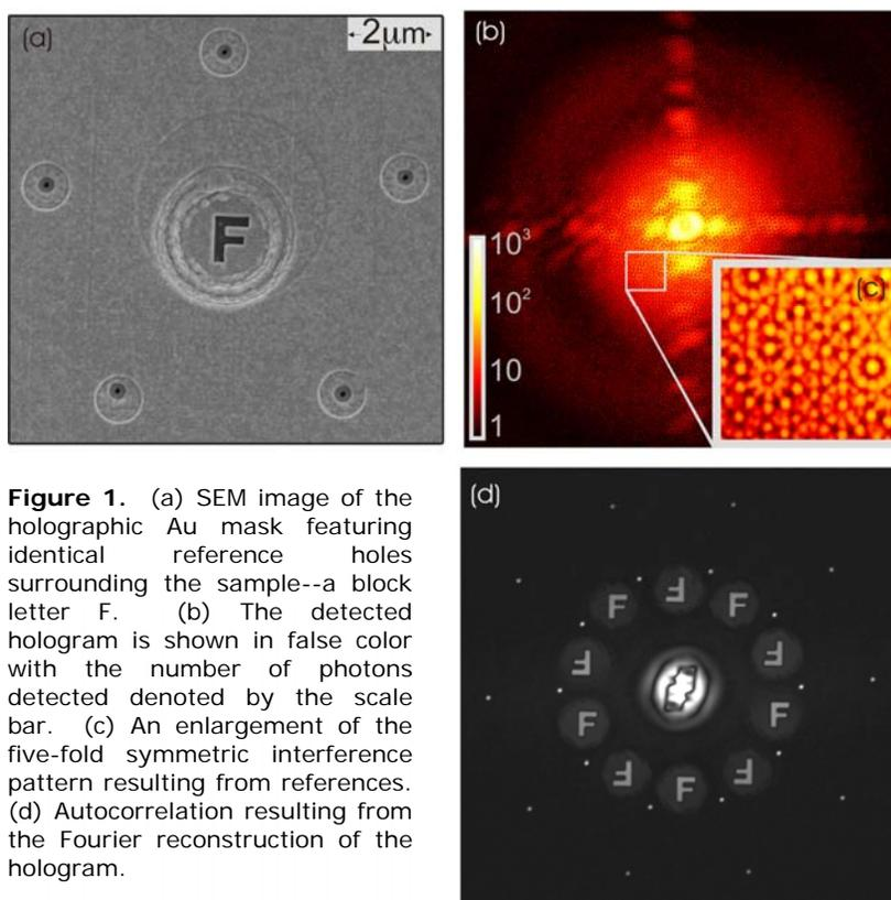
**Figure 1.** (a) SEM image of the holographic Au mask featuring identical reference holes surrounding the sample--a block letter F. (b) The detected hologram is shown in false color with the number of photons detected denoted by the scale bar. (c) An enlargement of the five-fold symmetric interference pattern resulting from references. (d) Autocorrelation resulting from the Fourier reconstruction of the hologram.
