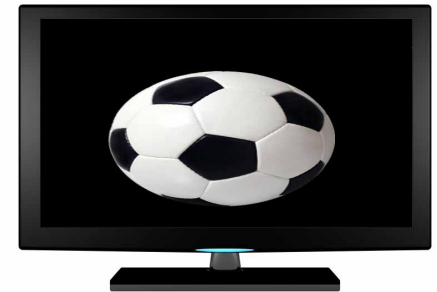
4:3 aspect ratio image on a screen set to an aspect ratio of 16:9
