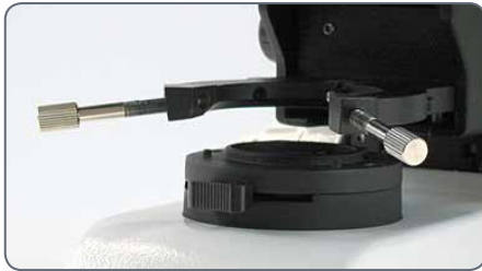
The holder of the condenser is open
