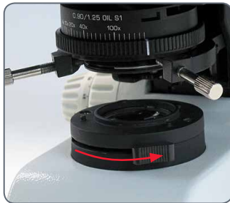
Close the Koehler field diaphragm
