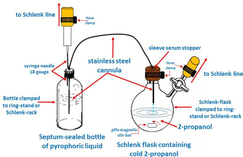
**Figure:** Schlenk line set-up to quench n-butyl lithium by dropwise addition into cold stirred 2-propanol. Ring-stand or rack clamps are not shown. The dry ice cold bath is not shown; nor the magnetic stir-plate.
