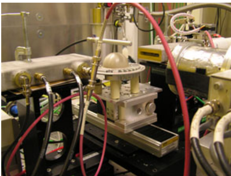
Figure 1: The EXAFS experimental setup. A Si(220) crystal was used in the monochromator with an energy resolution of about 1 eV. Sample powders were brushed onto sticky Kapton tape.
