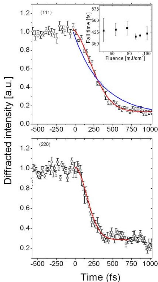
Fig. 1. (top) Time-resolved diffracted intensity for both (111) (top) and (220) (bottom) reflections. Red curves are Gaussian fits to the data, corresponding to 10-90 % fall times of 430 fs and 280 fs respectively. (inset) Fluence dependence of (111) time constant.
