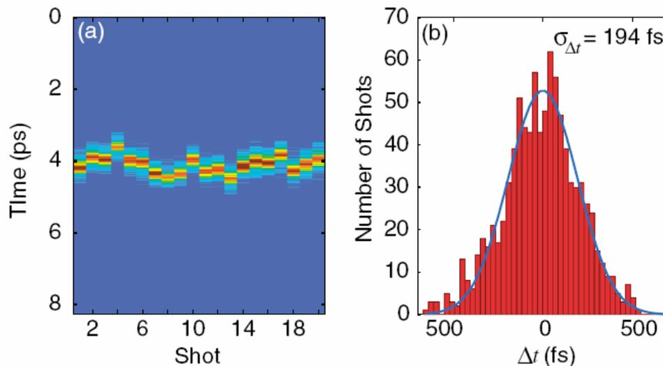
Fig. 2. (a) 20 consecutive single shot electron bunch measurements. The bright band in each column is the electro-optic signal, its location indicates the time of arrival of the electron bunch with respect to the laser probe pulse, and its width corresponds to the electron bunch duration. b) Normalized arrival time histogram of 1000 consecutive single shots.
