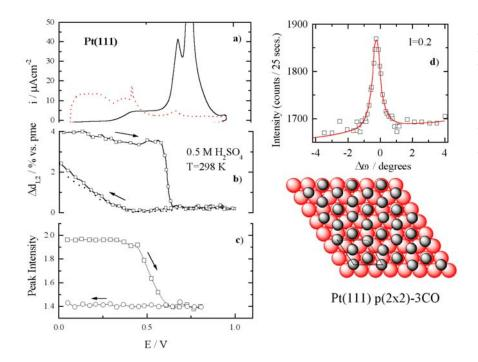
Figure 1. (a) CO stripping voltammetry on the Pt(111) surface in argon purged solution. (b) (---) Scattering intensity changes at (1, 0, 3.6) for the surface covered by CO<sub>ad</sub>; (c) Measured x-ray intensity at (1/2,1/2, 0.2) as а function of electrode potential for the same conditions as in (b). (d) A rocking scan through the (1/2,1/2, 0.2) position and model ideal for the p(2 x 2)-3CO structure.
