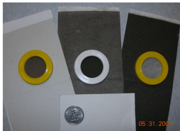
Figure 1. The good, the bad, and the ugly. Ambient airborne particulate matter captured on filters of woven silica fiber (large strips) and Teflon™ (round). Clean fiber filter at bottom for comparison. Take a deep breath?
