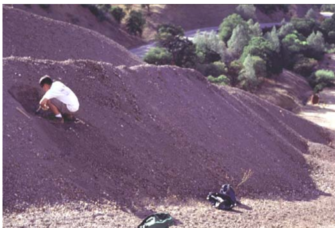
Figure 1. Dr. Christopher Kim collects a mine waste sample from the Oat Hill mercury mine in Northern California. The majority of mercury mine wastes at these sites are present as loose, unconsolidated piles, facilitating the transport of mercury-bearing material downstream into local watersheds.
