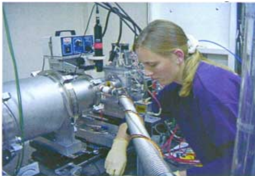
Kirsi Turbedsky (The Salk Institute) mounting a crystal on the low-angle single crystal diffraction instrument on BL4-2 during the SAXS/D workshop in March.
