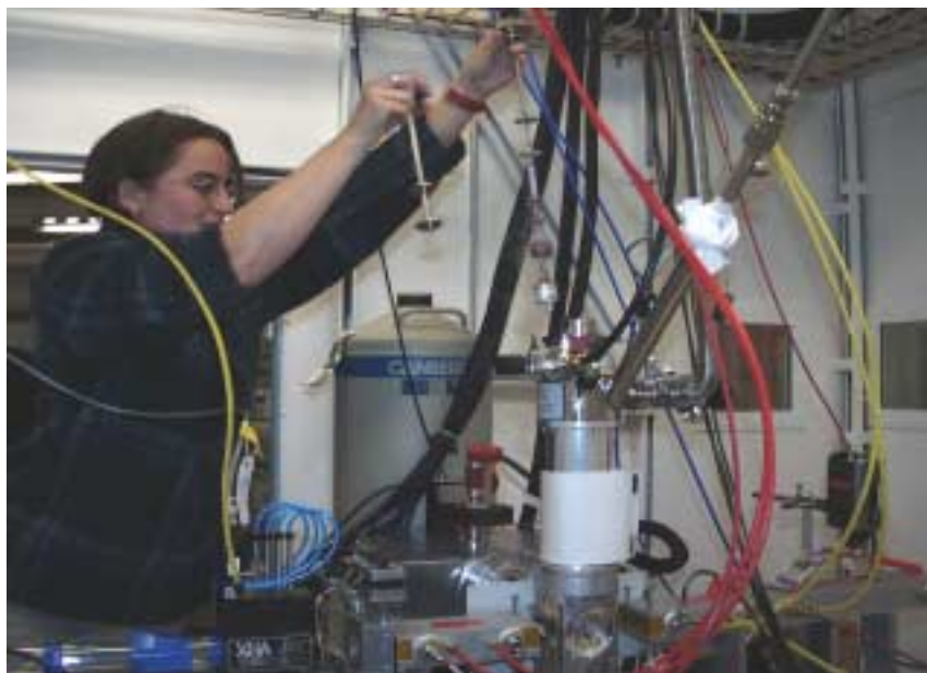
Shula Jaron, Oregon Graduate Institute (member of the N.J. Blackburn group) changing sample in the BL9-3 hutch during a commissioning run. In the foreground is the LHe cryostat into which the sample, at the end of the cryostat rod to the right, is being inserted. In the background is seen the 30-element Ge detector array.
