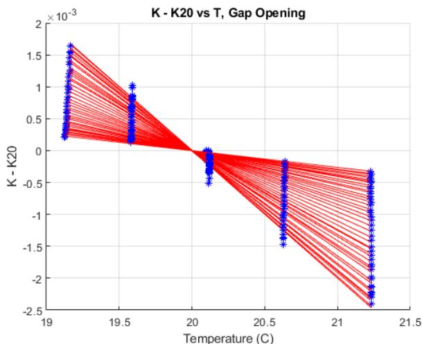
Figure 8: HXR undulator  $K$  as a function of temperature at all gaps as the gap is opening.
