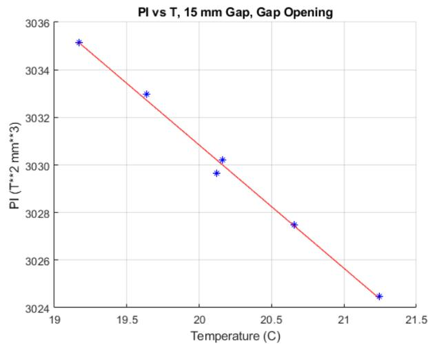
Figure 12: SXR phase shifter  $PI$  as a function of temperature at 15 mm gap.
