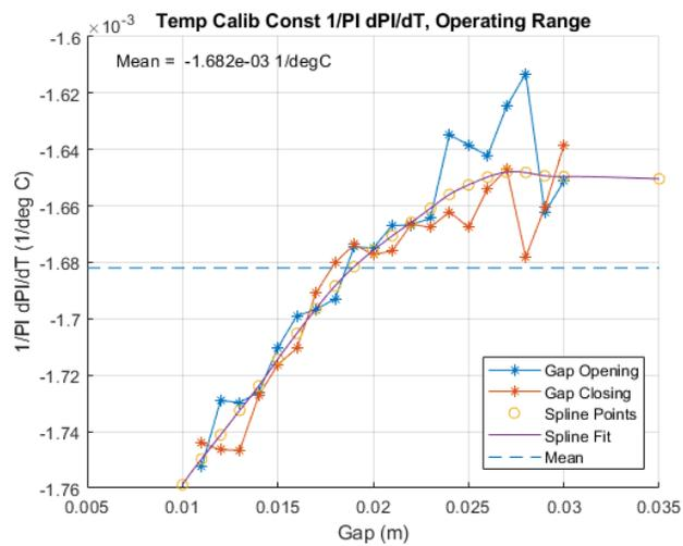
Figure 15: SXR phase shifter calibration constant  $1/PI dPI/dT$  as a function of gap.
