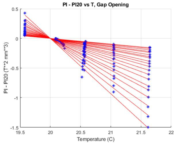
Figure 18: HXR phase shifter  $PI$  as a function of temperature at all gaps as the gap is opening.
