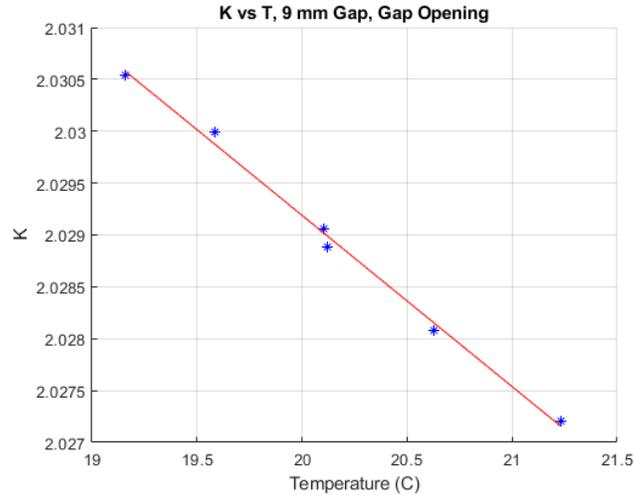
Figure 7: HXR undulator  $K$  as a function of temperature at 9 mm gap.
