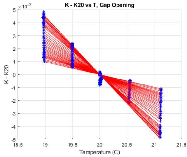
Figure 3: SXR undulator  $K$  as a function of temperature at all gaps as the gap is opening.
