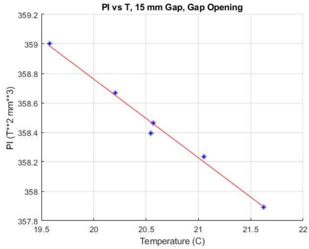
Figure 17: HXR phase shifter  $PI$  as a function of temperature at 15 mm gap.
