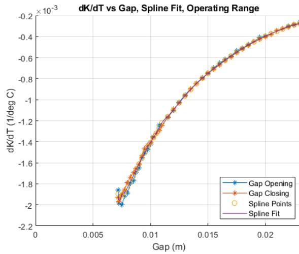
Figure 9: HXR undulator  $dK/dT$  as a function of gap. Values for both the gap opening and the gap closing are shown. Median values are used to generate points for a spline fit. The points for the fit and the fit itself are also shown.
