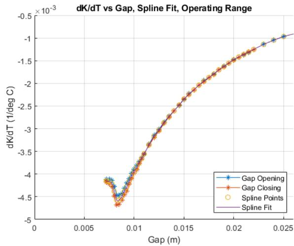
Figure 4: SXR undulator  $dK/dT$  as a function of gap. Values for both the gap opening and the gap closing are shown. Median values are used to generate points for a spline fit. The points for the fit and the fit itself are also shown.
