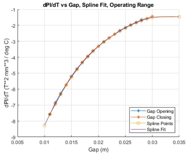
Figure 14: SXR phase shifter  $dPI/dT$  as a function of gap. Values for both the gap opening and the gap closing are shown. Median values are used to generate points for a spline fit. The points for the fit and the fit itself are also shown.
