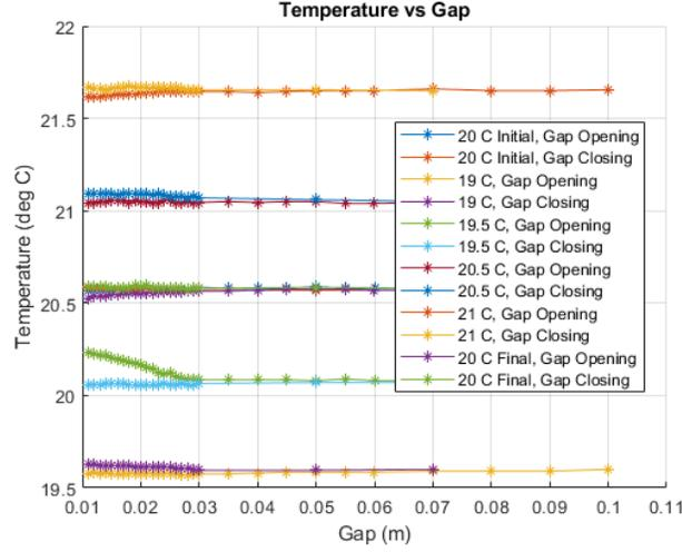
Figure 16: Temperature of the HXR phase shifter during the test.
