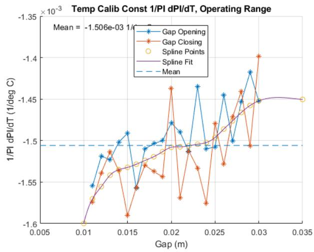
Figure 20: HXR phase shifter calibration constant  $1/PI \frac{dPI}{dT}$  as a function of gap.
