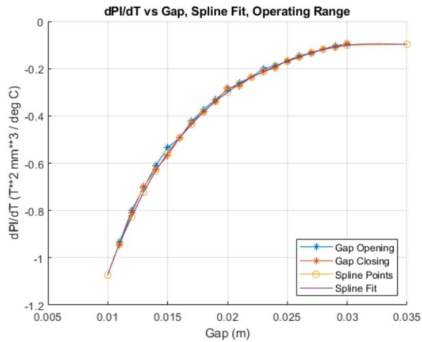
Figure 19: HXR phase shifter  $dPI/dT$  as a function of gap. Values for both the gap opening and the gap closing are shown. Median values are used to generate points for a spline fit. The points for the fit and the fit itself are also shown.
