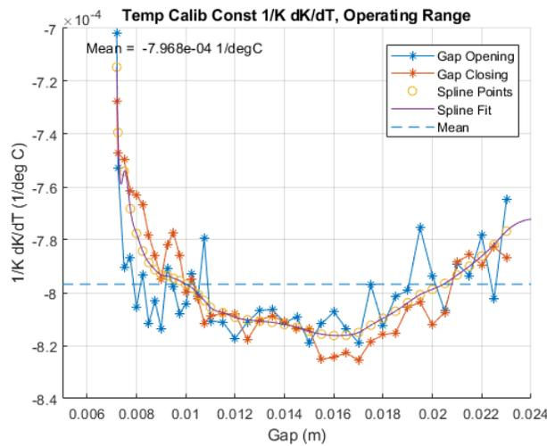
Figure 10: HXR undulator calibration constant  $1/K dK/dT$  as a function of gap.
