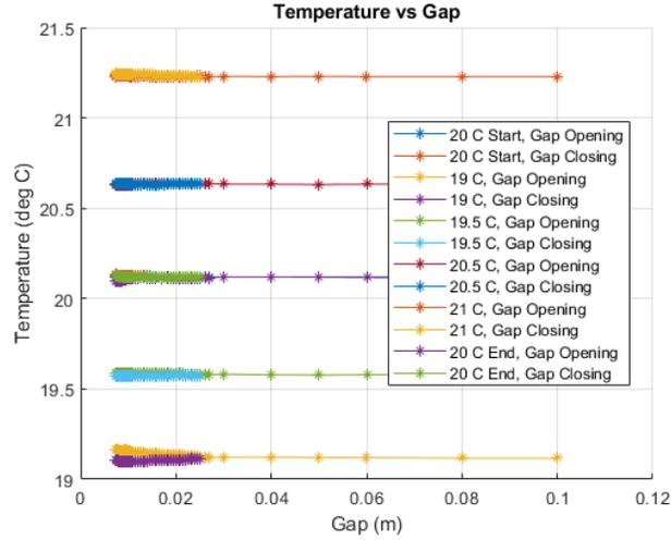
Figure 6: Temperature of the HXR undulator during the test.
