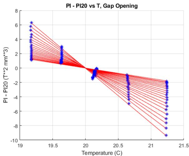
Figure 13: SXR phase shifter  $PI$  as a function of temperature at all gaps as the gap is opening.
