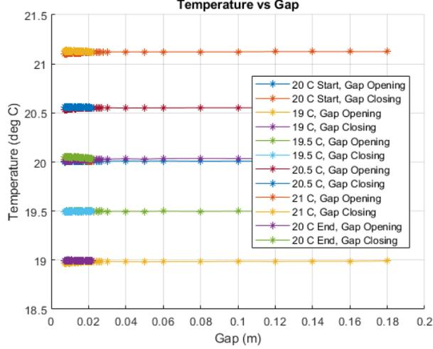
Figure 1: Temperature of the SXR undulator during the test.
