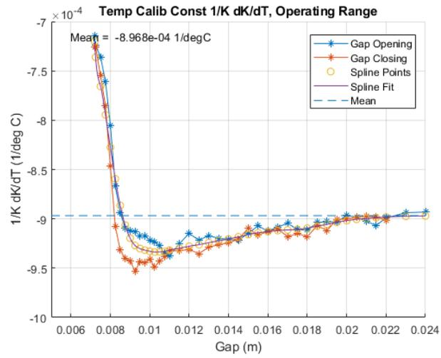
Figure 5: SXR undulator calibration constant  $1/K dK/dT$  as a function of gap.
