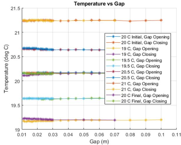
Figure 11: Temperature of the SXR phase shifter during the test.
