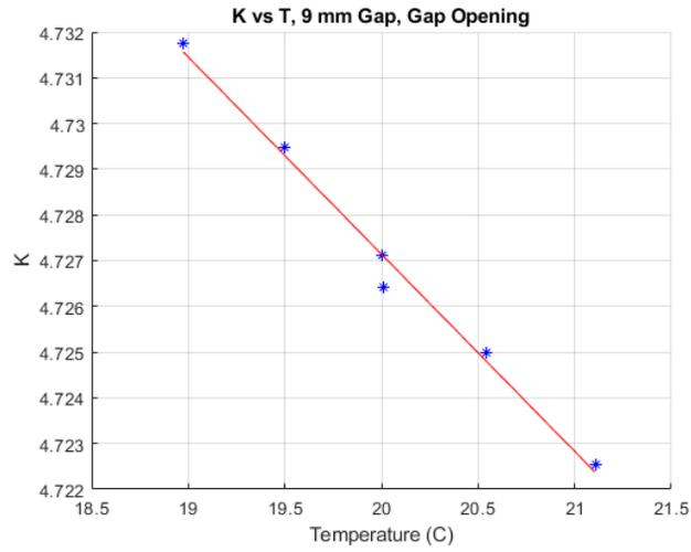
Figure 2: SXR undulator  $K$  as a function of temperature at 9 mm gap.
