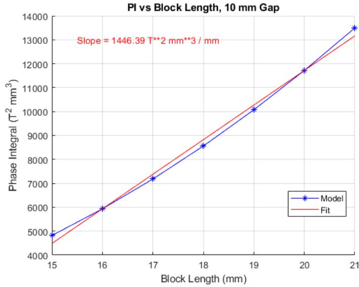
Figure 10: Phase integral as a function of block length at 10 mm gap. The block height is 25 mm and the block width is 65 mm.
