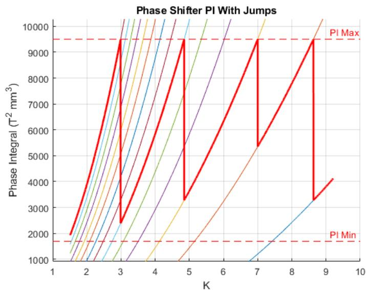
Figure 23: Phase shifter jumps for an interspace with an undulator in each neighboring cell.
