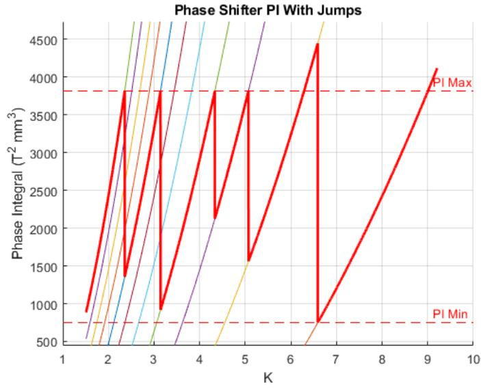
Figure 4: An LCLS-II SXR phase shifter can not be used to cover the range of  $K$  values of LCLS-II-HE.
