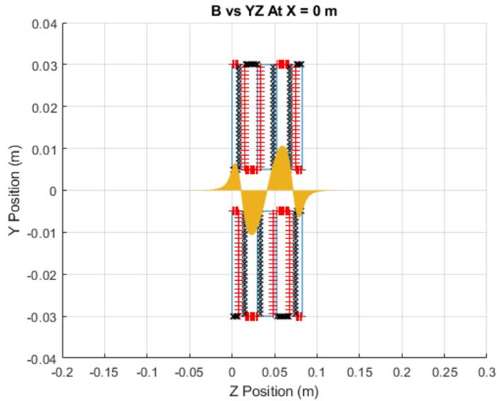
Figure 6: Model of the phase shifter in which the magnet blocks are replaced by magnetic charges.
