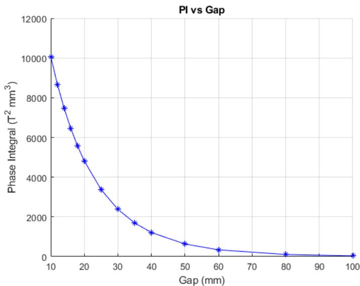
Figure 21: Phase integral as a function of gap.
