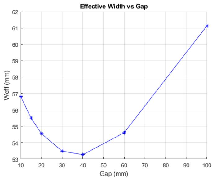
Figure 29: Phase shifter effective width as a function of gap.
