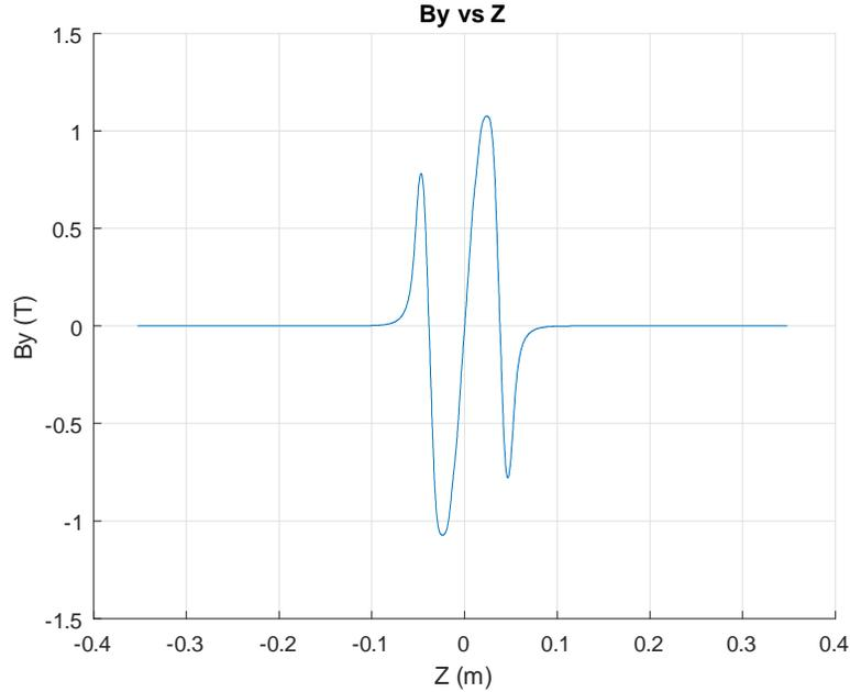
Figure 27: The vertical field  $B_y$  as a function of  $z$  on the magnetic axis with 10 mm gap.
