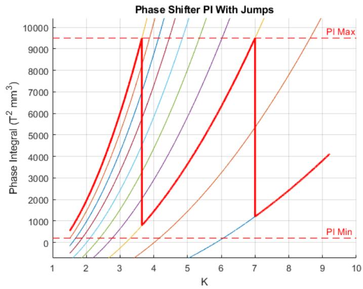
Figure 5: The proposed LCLS-II-HE phase shifters cover the range of undulator  $K$  values.
