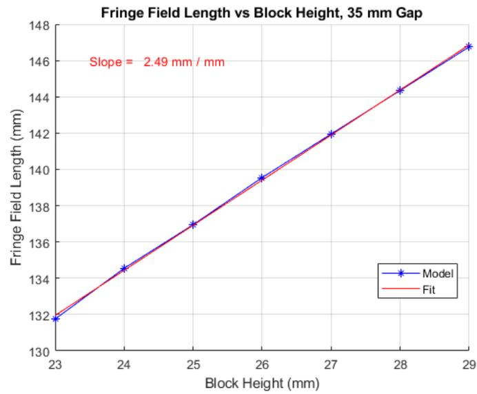
Figure 17: Fringe field length as a function of block height.
