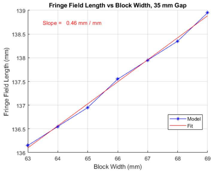
Figure 18: Fringe field length as a function of block width.
