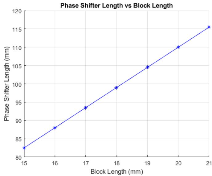
Figure 12: Phase shifter length as a function of block length.
