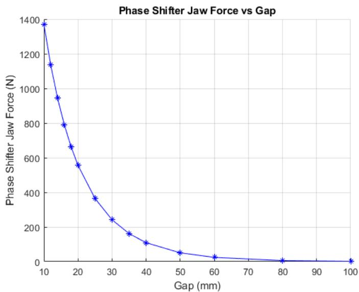
Figure 30: Force on a phase shifter jaw as a function of gap.
