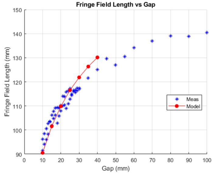
Figure 8: Length of the fringe field from SXPS-16336 and from the model.
