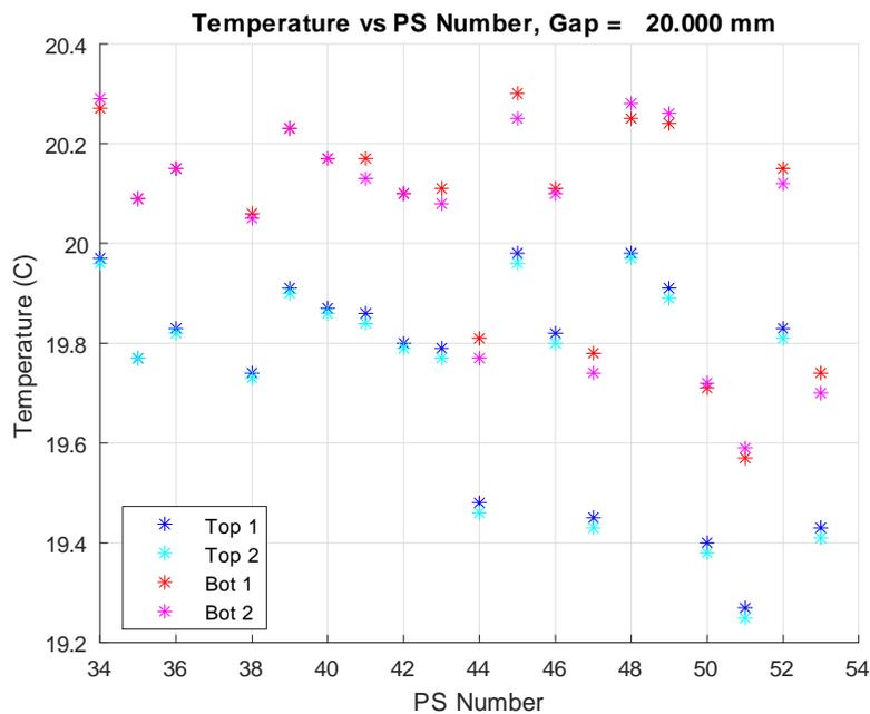
Figure 31: Temperature of the upper and lower jaws of the SXR phase shifters measured during their calibration.
