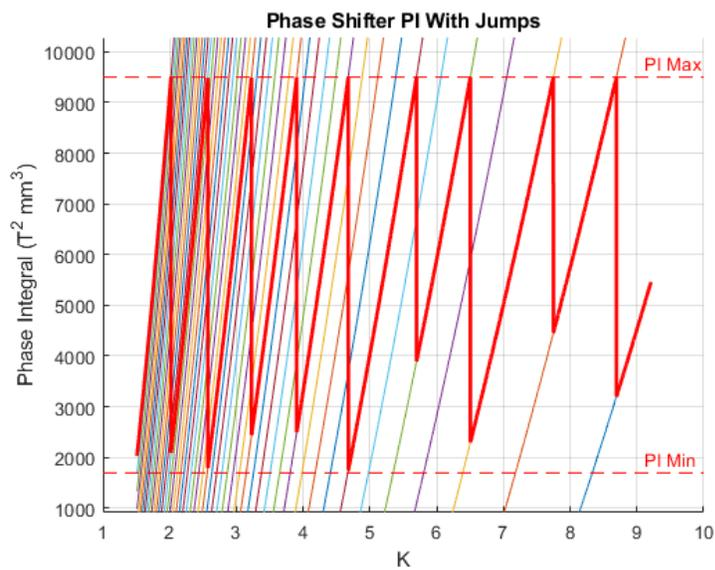
Figure 24: Phase shifter jumps when correcting for the drift in a cell without an undulator.
