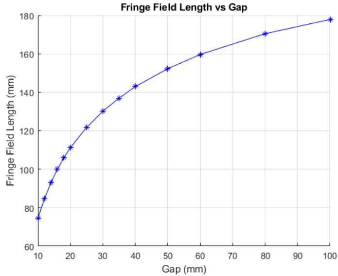
Figure 22: Fringe field length as a function of gap.
