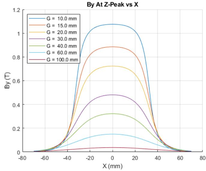
Figure 28: Field  $B_y$  as a function of  $x$  at several gaps at a  $z$ -position where the field is maximal.
