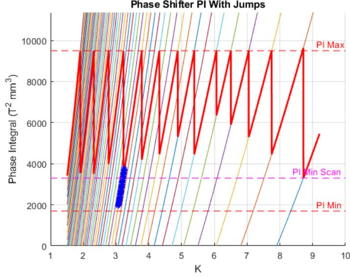
Figure 26: Phase shifter settings during a 10% energy scan for a cell with no undulator.
