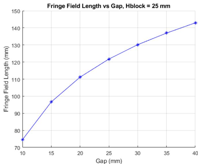
Figure 15: Fringe field length as a function of phase shifter gap.
