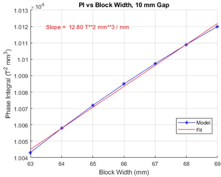
Figure 14: Phase integral as a function of block width at 10 mm gap. The block length is 19 mm and the block height is 25 mm.
