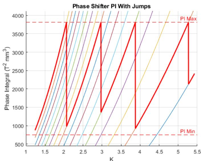
Figure 3: The LCLS-II SXR phase shifters have a series of  $2\pi n$  jumps to cover the range of undulator  $K$  values.
