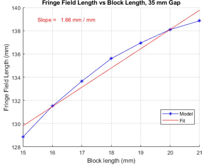
Figure 16: The fringe field length depends on the block length.
