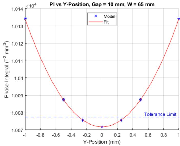
Figure 20: Phase integral as a function of  $y$  with  $x = 0$ .
