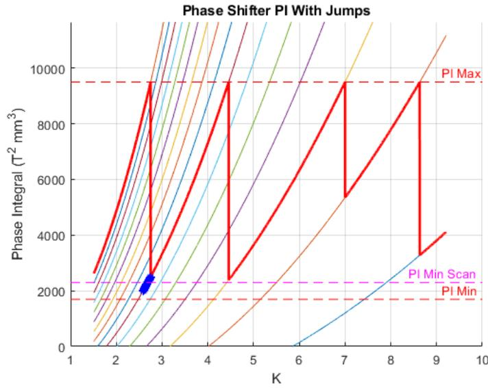
Figure 25: During an energy scan, the phase integrals can follow a curve with a given additive multiple of  $2\pi$ . The minimum phase integral setting for the scan keeps the phase integral larger than the actual minimum.
