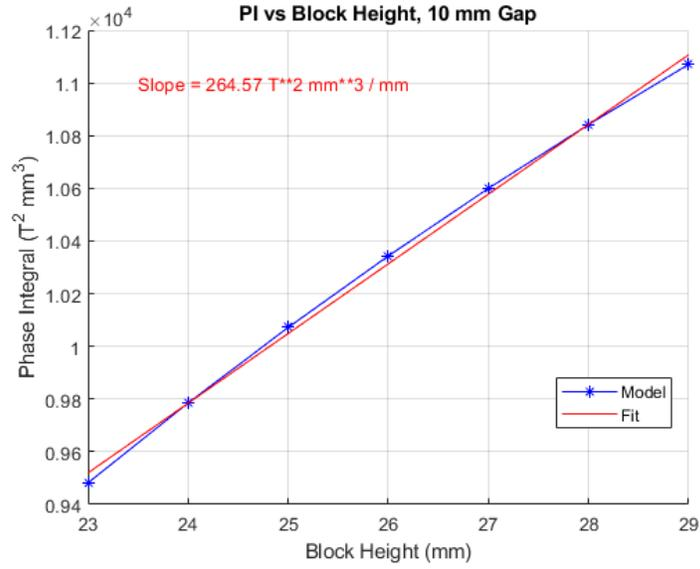
Figure 13: Phase ingegral as a function of block height at 10 mm gap. The block length is 19 mm and the block width is 65 mm.
