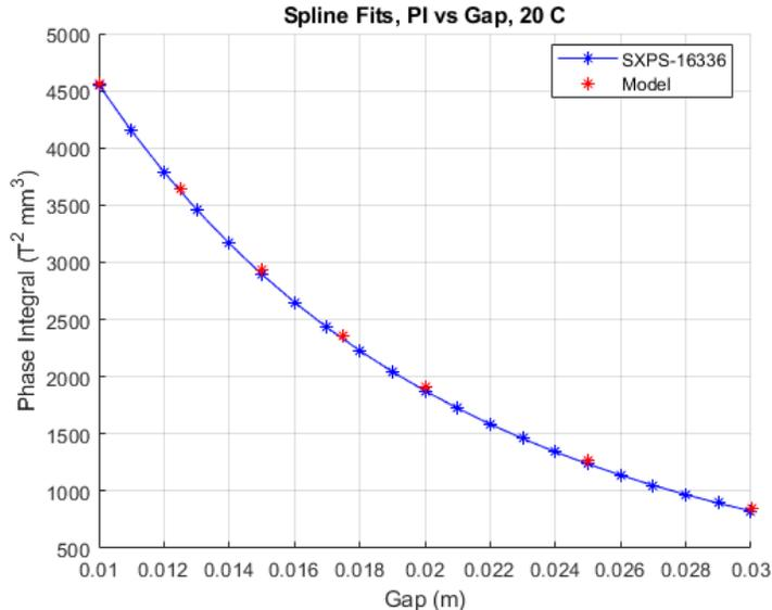
Figure 7: Phase integral as a function of gap for a measured phase shifter and the model.
