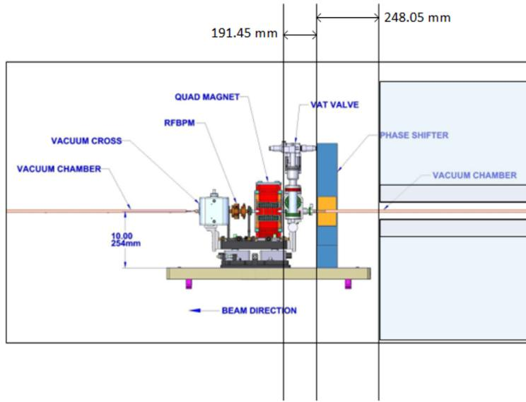
Figure 2: Interspace layout of the SXR-HE line. The dimensions show the distance from the edge of the phase shifter to the quadrupole and undulator.
