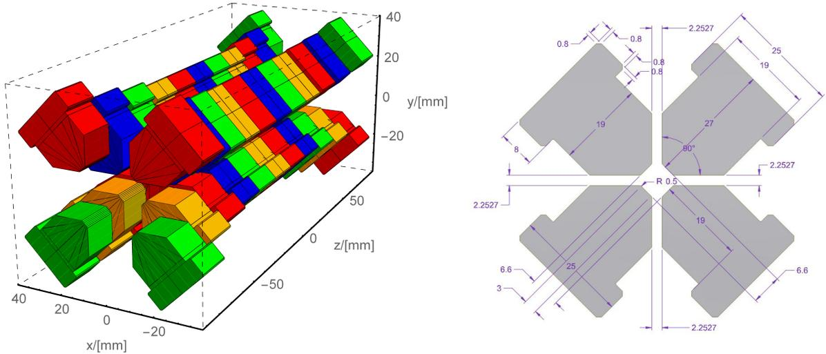
(a) RADIA model (One core period chosen for better visualization) (b) Dimensioned cross section of closed gap core magnet arrangement (F. Peters) used in modelling
