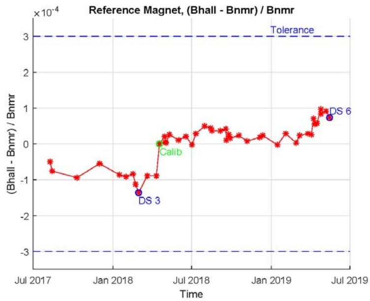
Figure 10: Comparison of Hall probe to NMR measurements of a reference dipole over time.
