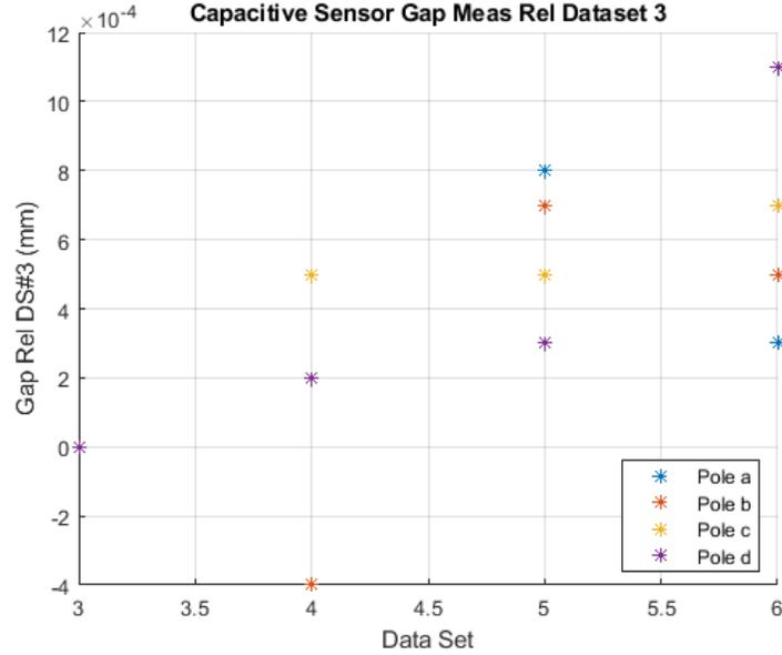
Figure 8: The change in undulator gap relative to dataset 3 is typically below one micron. A gap of 46.6 mm was used for these measurements.
