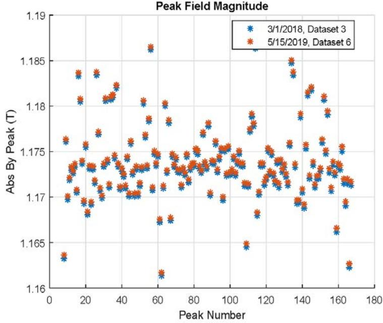
Figure 2:  $B_y$  peak fields for the measurements before and after the latest fourteen months in storage.
