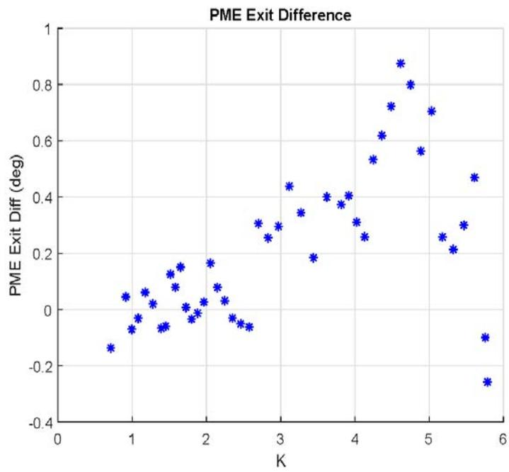
Figure 13: Difference in the spline fits to the phase matching error at the undulator exit as a function of  $K$ .
