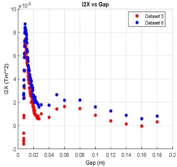
Figure 16: Comparison of the measurements of the second integral of  $B_x$ .
