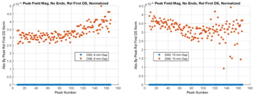
Figure 9: Difference in the absolute value of the peak fields, dataset 6 minus dataset 3, normalized to the dataset 3 peak fields. The left plot is for 9 mm gap, and the right plot is for 15 mm gap.
