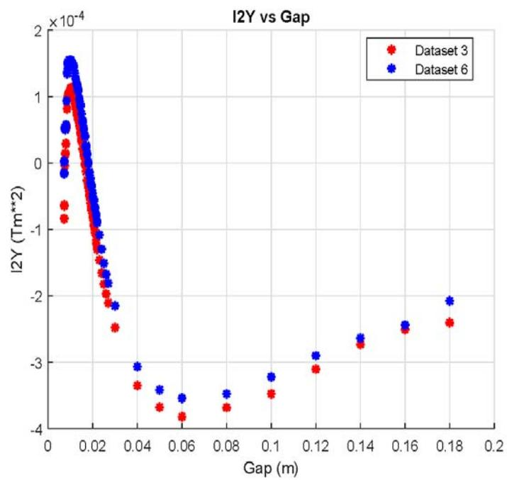
Figure 17: Comparison of the measurements of the second integral of  $B_y$ .
