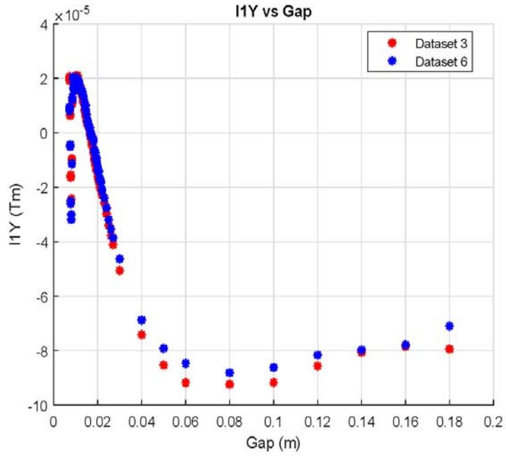
Figure 15: Comparison of the measurements of the first integral of  $B_y$ .
