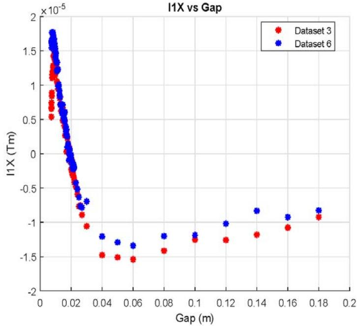
Figure 14: Comparison of the measurements of the first integral of  $B_x$ .
