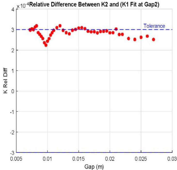
Figure 7: Difference in the K value before and after storage as a function of gap.
