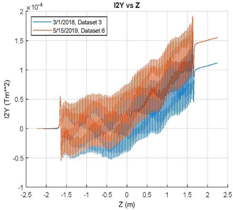
Figure 5: Comparison of the second integral of  $B_y$ .
