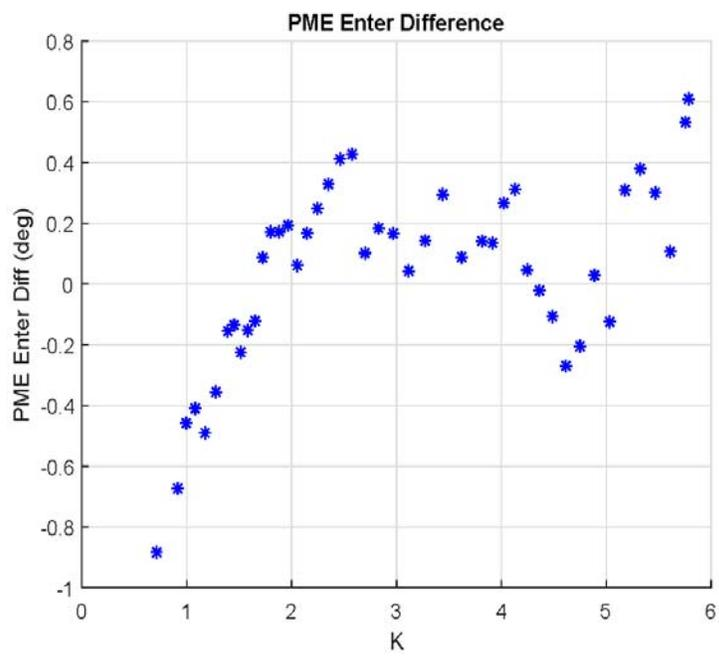
Figure 12: Difference in the spline fits to the phase matching error at the undulator entrance as a function of K.
