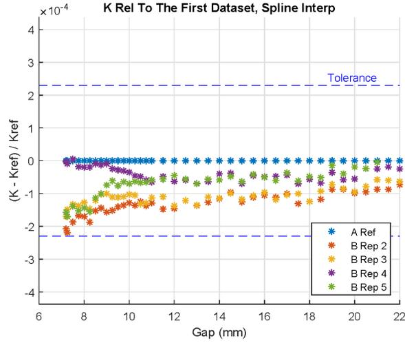
Figure 11: Comparison of measurements made in the B position to the reference measurement made in the A position.
