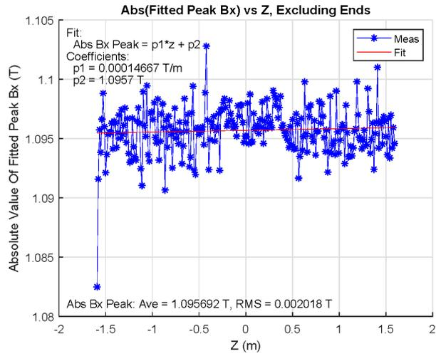
Figure 9: The magnitude of the peak fields at 7.2 mm gap in the A mounting position.
