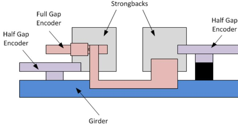
Figure 2: Schematic of the hard x-ray undulator and its encoders.
