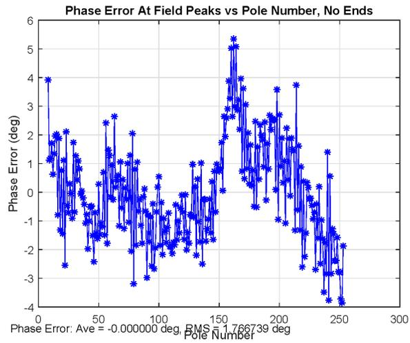
Figure 10: Phase errors at 7.2 mm gap in the A mounting position.
