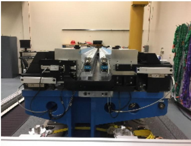
Figure 1: Photo showing the full gap encoder and the half gap encoders at the upstream end of HXU-017.
