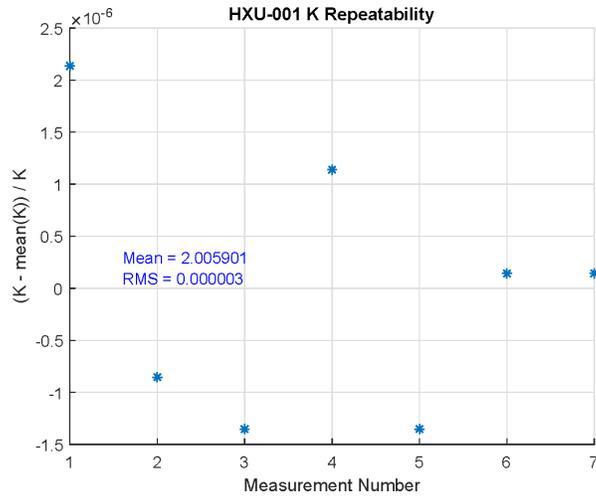
Figure 7: This plot shows the repeatability of the K value calculated from seven measurements taken without changing the undulator gap.
