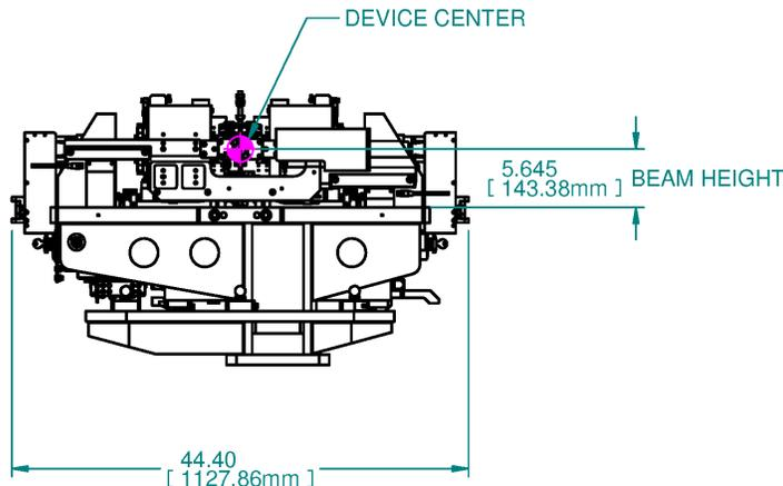
Figure 6: Drawing of the undulator as seen from the downstream end.
