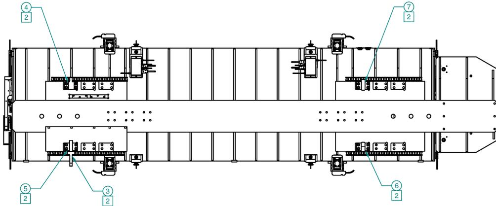
Figure 4: Bottom view of the HXU girder. The surfaces that go into the kinematic mount are labeled. The drawing shows the mounting surfaces in the C position.
