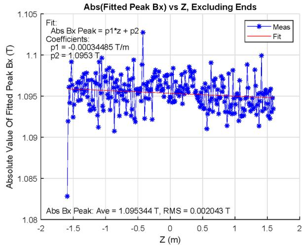
Figure 15: The magnitude of the peak fields at 7.2 mm gap in the C mounting position.
