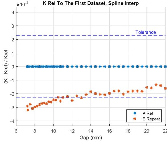
Figure 17: Repeat measurements in the B position compared to the reference measurements in the A position.
