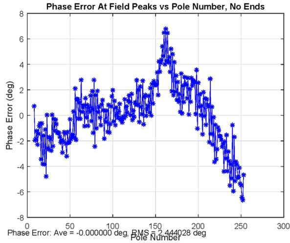
Figure 13: Phase errors at 7.2 mm gap in the B mounting position.
