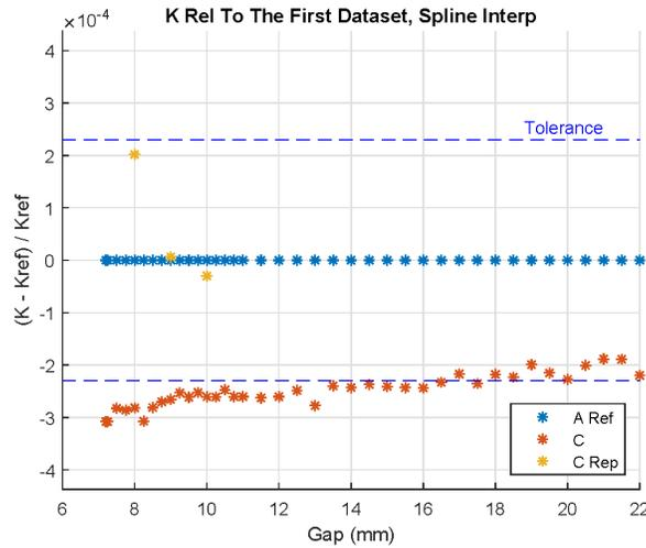
Figure 14: Measurements in the C position relative to the reference measurement in the A position.
