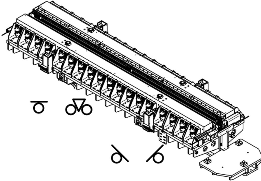
Figure 5: The HXU rests on a kinematic mount. This is illustrated by the V's and flat below the undulator.
