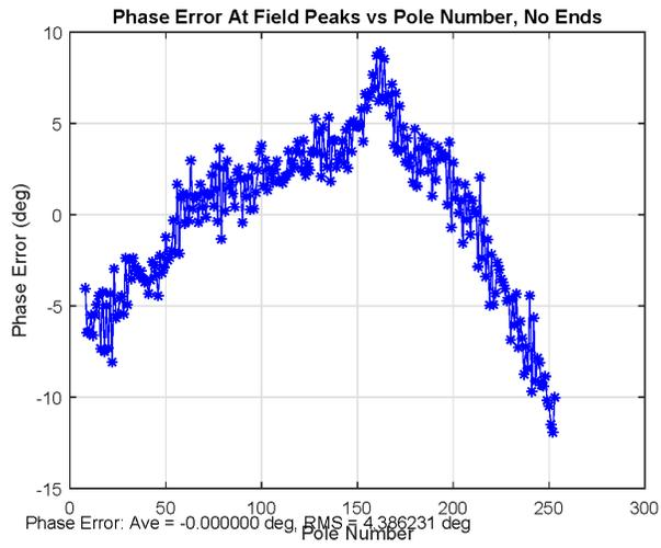
Figure 16: Phase errors at 7.2 mm gap in the C mounting position.
