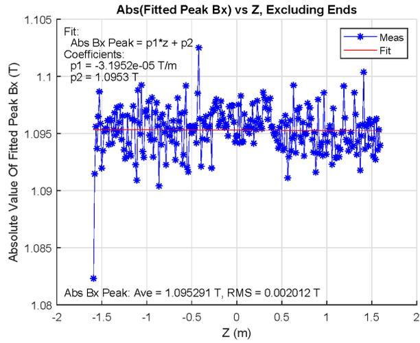
Figure 12: The magnitude of the peak fields at 7.2 mm gap in the B mounting position.
