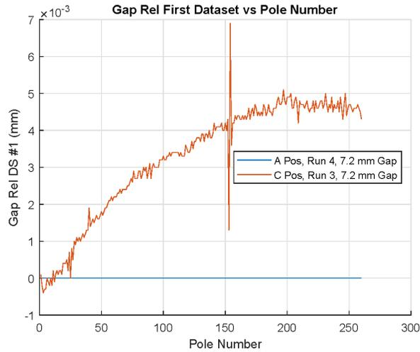
Figure 18: In the C position the gap gets systematically larger than in the A position for the same readings of the half gap encoders.
