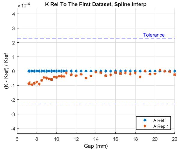
Figure 8: The two measurements in the A position repeated within tolerance.
