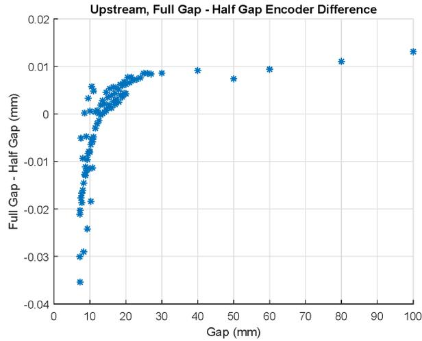
Figure 3: Difference between the full gap encoder reading and the sum of the half gap encoder readings as a function of gap.
