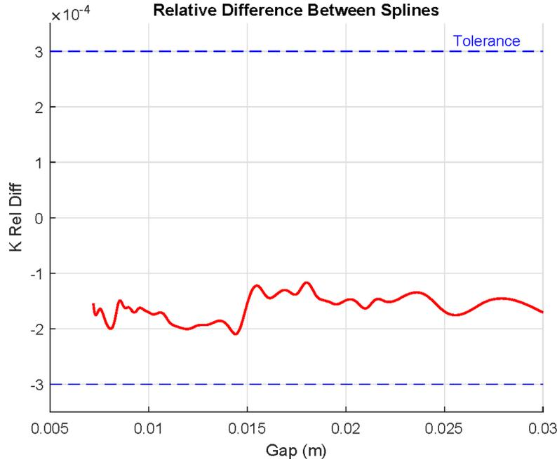
Figure 7: Difference in the K value before and after storage as a function of gap.
