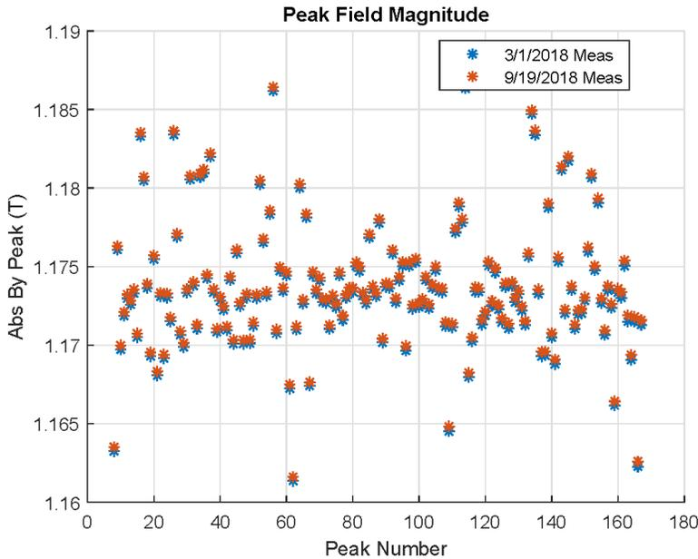
Figure 2:  $B_y$  peak fields for the measurements before and after the second six months in storage.
