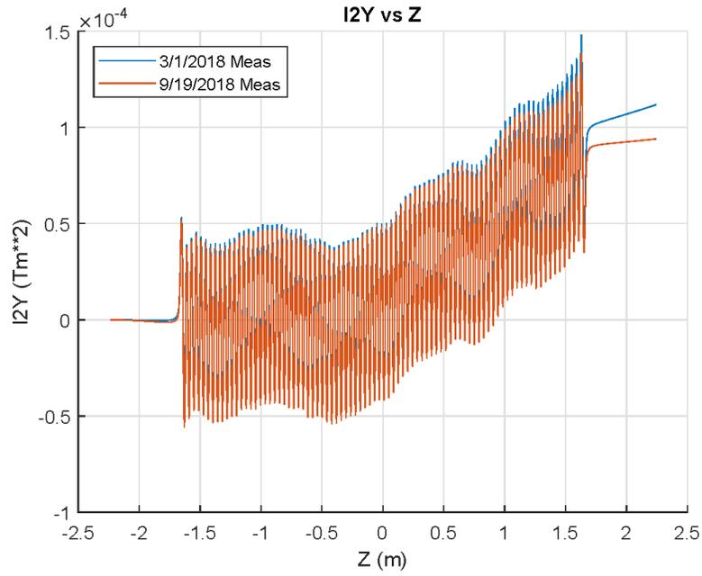
Figure 5: Comparison of the second integral of  $B_y$ .
