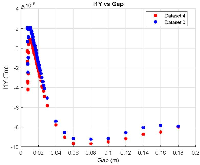
Figure 12: Comparison of the measurements of the first integral of  $B_y$ .
