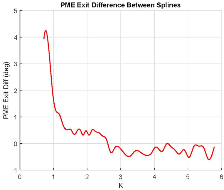
Figure 10: Difference in the spline fits to the phase matching error at the undulator exit as a function of K.
