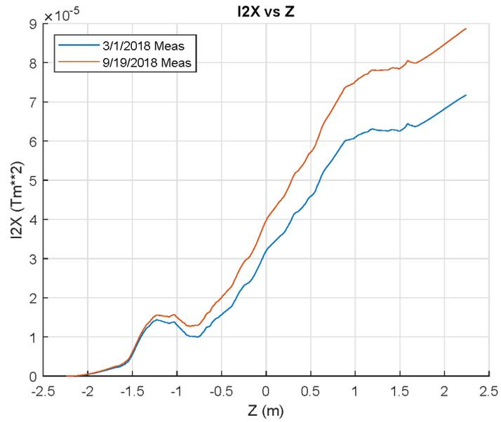
Figure 4: Comparison of the second integral of  $B_x$ .
