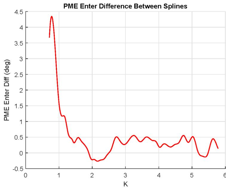
Figure 9: Difference in the spline fits to the phase matching error at the undulator entrance as a function of  $K$ .
