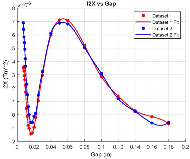
Figure 14: Comparison of the measurements of the second integral of  $B_x$ .
