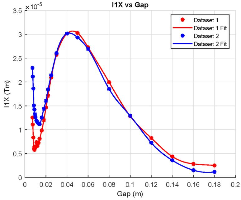
Figure 12: Comparison of the measurements of the first integral of  $B_x$ .
