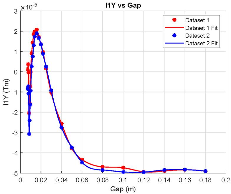
Figure 13: Comparison of the measurements of the first integral of  $B_y$ .
