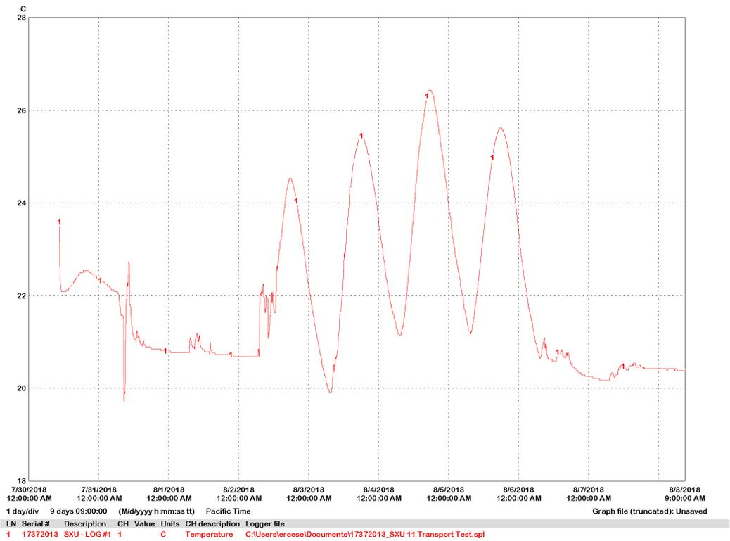
Figure 1: Temperature of SXU-011 during the transportation test.
