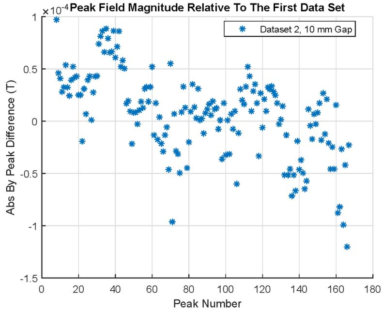
Figure 3: Difference of the peak field magnitudes after the transportation test compared to before the test.
