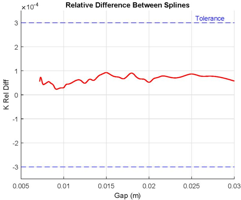
Figure 7: Difference in the K value before and after transport as a function of gap.
