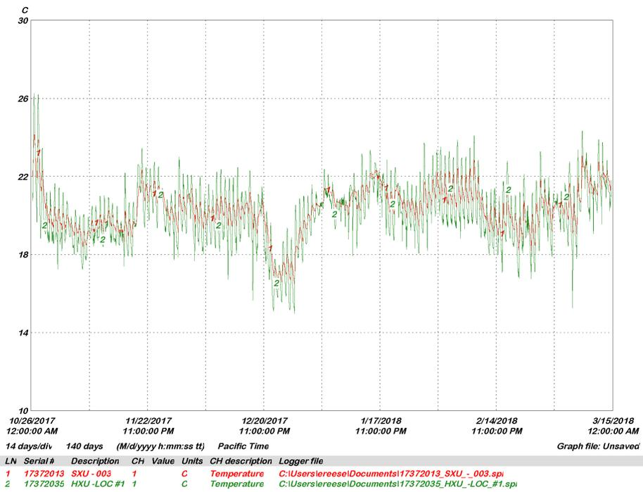
Figure 1: Undulator temperature and ambient temperature in the storage area.
