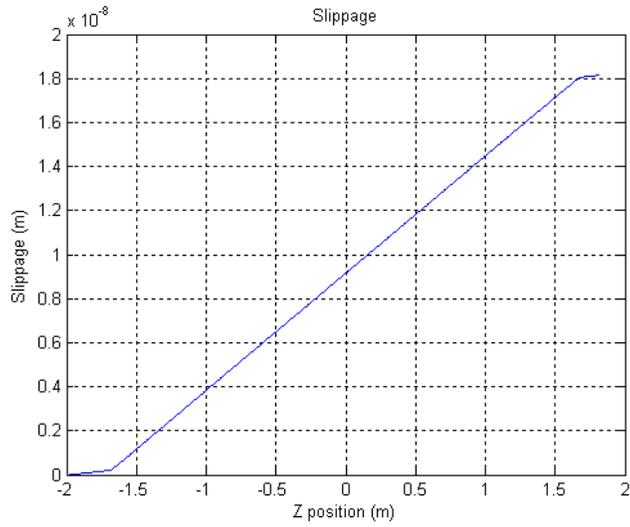
Figure 11: The slippage change is small outside the undulator and large in the undulator where the slope terms contribute.
