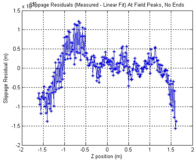
Figure 12: Residuals from a linear fit to the slippage in the undulator.
