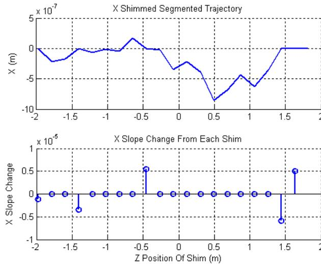
Figure 4: Shims are combined leaving an imperfect but acceptable trajectory. The combinations result in a great reduction in the number of shims.
