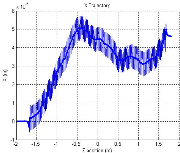
Figure 1: Calculated x trajectory from the measured fields.
