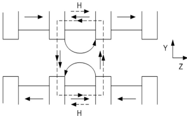
Figure 21: The dashed line shows the path used in the calculation of Ampere's law. The solid arrows show  $B$ . The two dashed arrows show  $H$  in the permanent magnet blocks.
