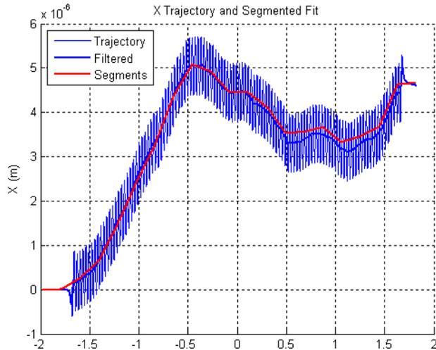
Figure 2: Line segments are fit to the trajectory and joined, making the segmented trajectory.
