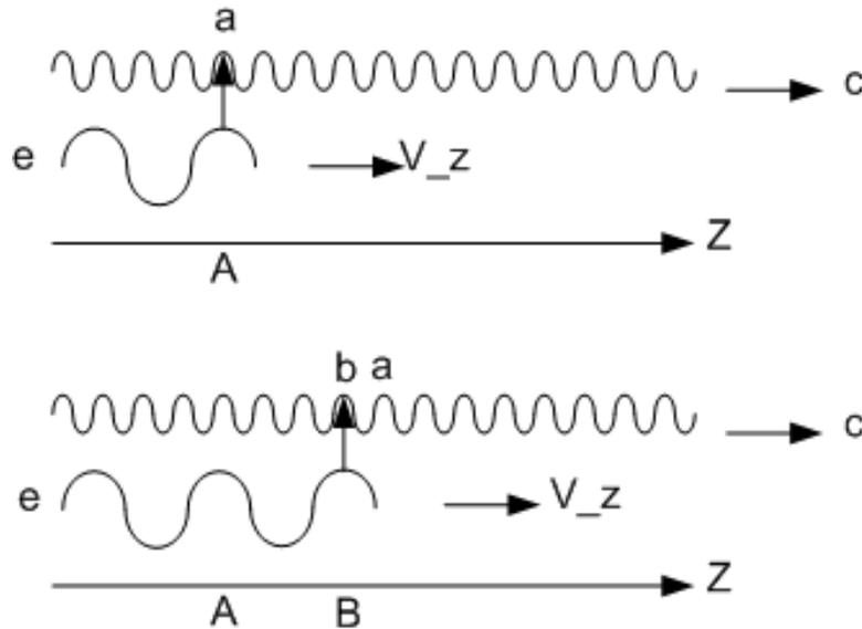
Figure 10: The upper figure shows an electron at position "A" adding photon "a" to the radiation wave. The lower figure shows the situation after the electron has moved one undulator period to position "B". The electron adds photon "b", which is behind "a" because "a" is moving forward faster than the electron.
