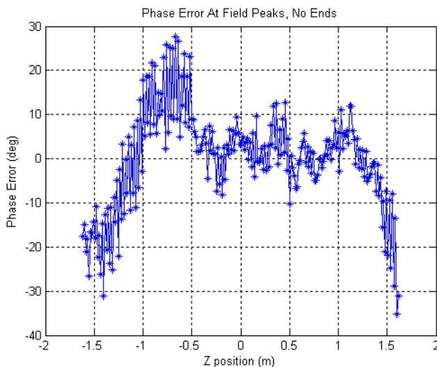
Figure 13: Plot of phase errors at the undulator poles.
