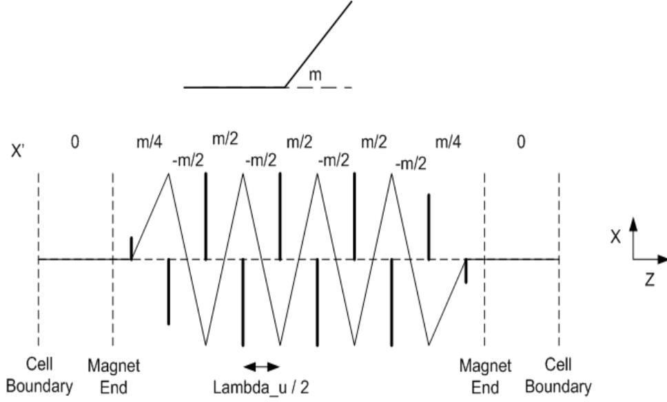
Figure 25: The undulator field is replaced by impulsive forces. The upper part of the figure shows the effect of a short pole giving the trajectory a slope change equal to that of a full strength pole. The lower part of the figure shows the model of the undulator field replaced by the impulsive forces. The trajectory is shown and the trajectory slopes are given.
