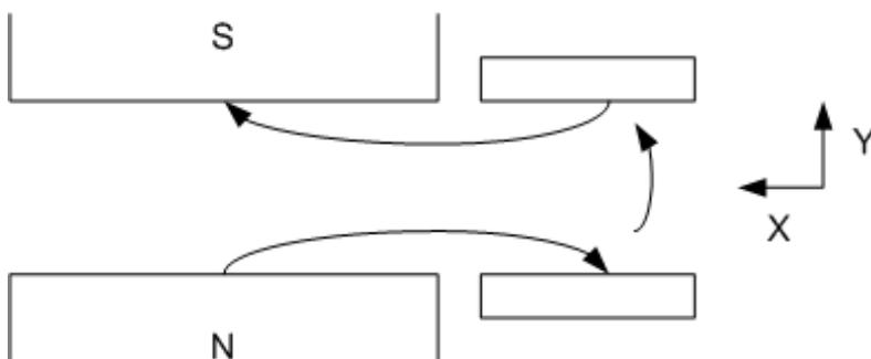
Figure 7: The  $x$  trajectory shims are placed on both the upper and lower poles to cancel the horizontal field.
