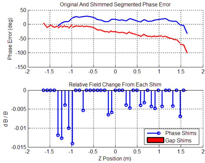
Figure 19: Phase shims are applied in all segments where the phase error increases above a threshold value.
