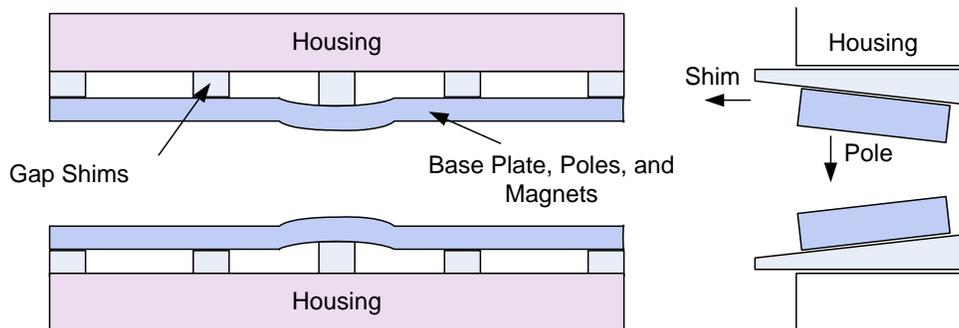
Figure 18: Gap shims are used to increase or decrease the gap. The magnetic field in the gap changes, which in turn changes the phase.
