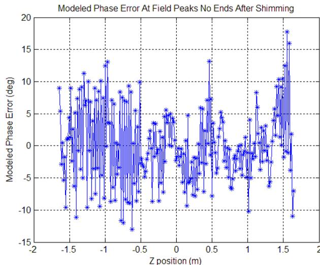
Figure 22: The magnetic effect of the phase error shims are calculated and superimposed on the measured field. The phase errors are then calculated, resulting in this prediction of the phase errors after shimming.
