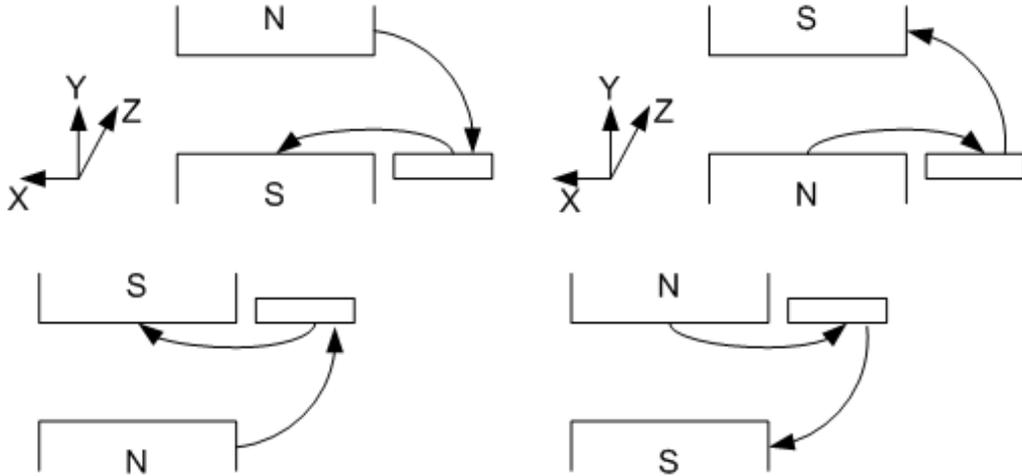
Figure 8: Shims for the  $y$  trajectory are placed on succeeding sets of poles.
