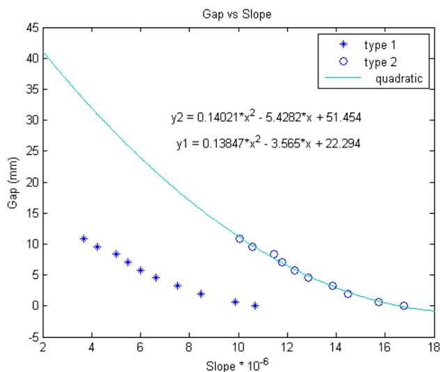
Figure 6: The distance between the shim and a pole is calculated using a fit to measured distance vs slope change data.
