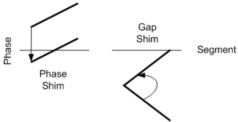
Figure 17: Phase shims cause a rapid phase decrease moving the segment downward. Gap shims change the slope of a segment.
