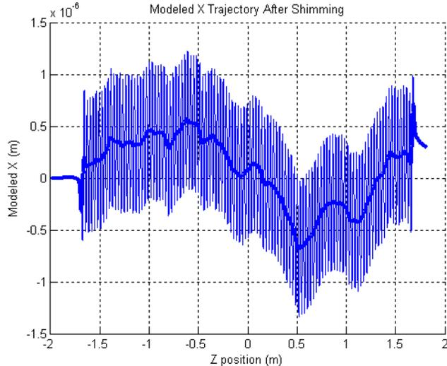
Figure 9: The required shim fields are added to the measured fields and the resulting trajectory is calculated giving the predicted shimmed trajectory.
