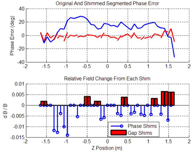
Figure 20: Gap shims are applied to bring the phase errors to zero.
