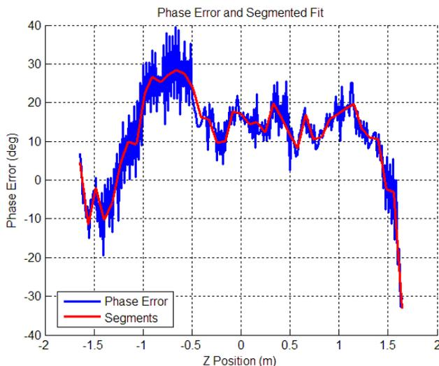
Figure 15: The phase error is fit with line segments giving the segmented phase error.
