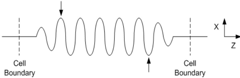
Figure 24: Electron trajectory with the reference poles marked with arrows. The phase from the cell boundary to the first reference pole, the phase between reference poles, and the phase from the second reference pole to the far cell boundary must all be set to required values.
