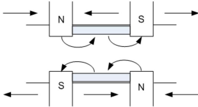
Figure 16: Phase shims shunt flux out of the gap and weaken two poles.
