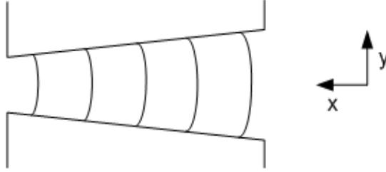
Figure 23: The poles of the LCLS undulators are canted to produce a field which varies with  $x$ .
