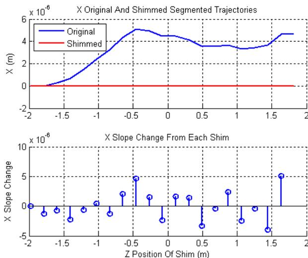
Figure 3: One shim per segment is calculated to make the segmented trajectory flat. The required slope changes are shown.
