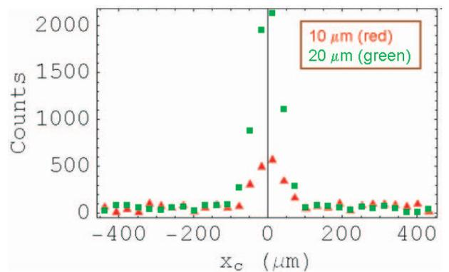
FIG. 4: The signal strength for BFW with diameter of  $10 \mu\text{m}$  (red) and  $20 \mu\text{m}$  (green).
