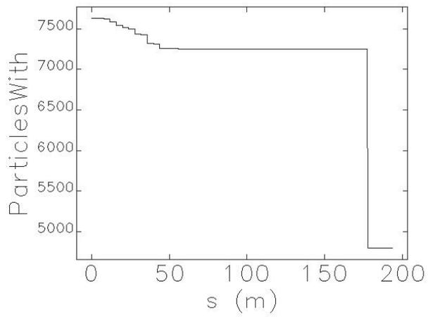
FIG. 5: Halo electrons loss along the undulator.
