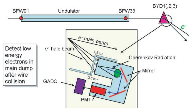
FIG. 1: Layout of the threshold Cherenkov Counter in the main dump line after the undulator.
