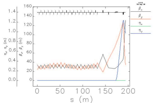
FIG. 2: Twiss parameters for the undulator and the main beam dump line.
