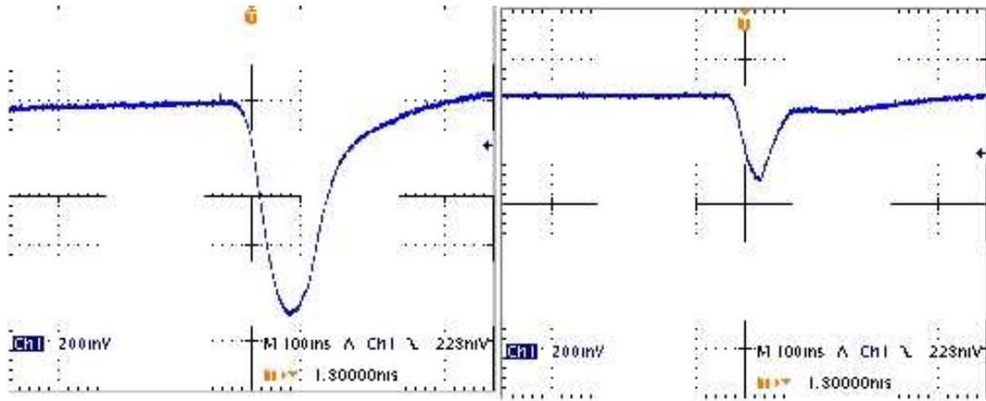
Figure 4: Current Spikes when turning off Power Supply of MCOR Calibration Stand;
