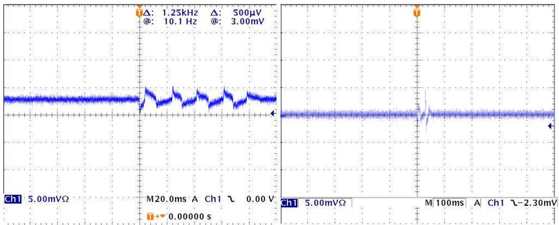
Figure 5: Current Spikes when turning off bulk power supply of MCOR 12;
