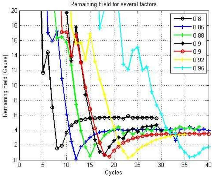
Figure 2: Remaining integrated field after cycles of degaussing.
