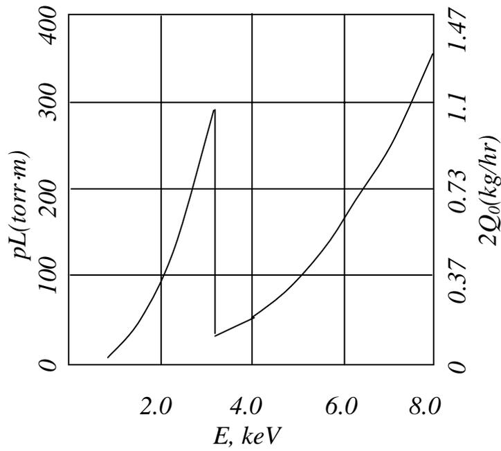
Fig. 2 The argon line density required to produce a  $10^4$  attenuation at various photon energies (left scale), and the un-inhibited exhaust from two 3-mm diameter orifices from the attenuation cell, for the length of the attenuation cell  $L= 6$  m (right scale). For the attenuation  $A=100$  the vertical scale should be divided by a factor of 2; for the attenuation  $A=10$ , the vertical scale should be divided by a factor of 4.
