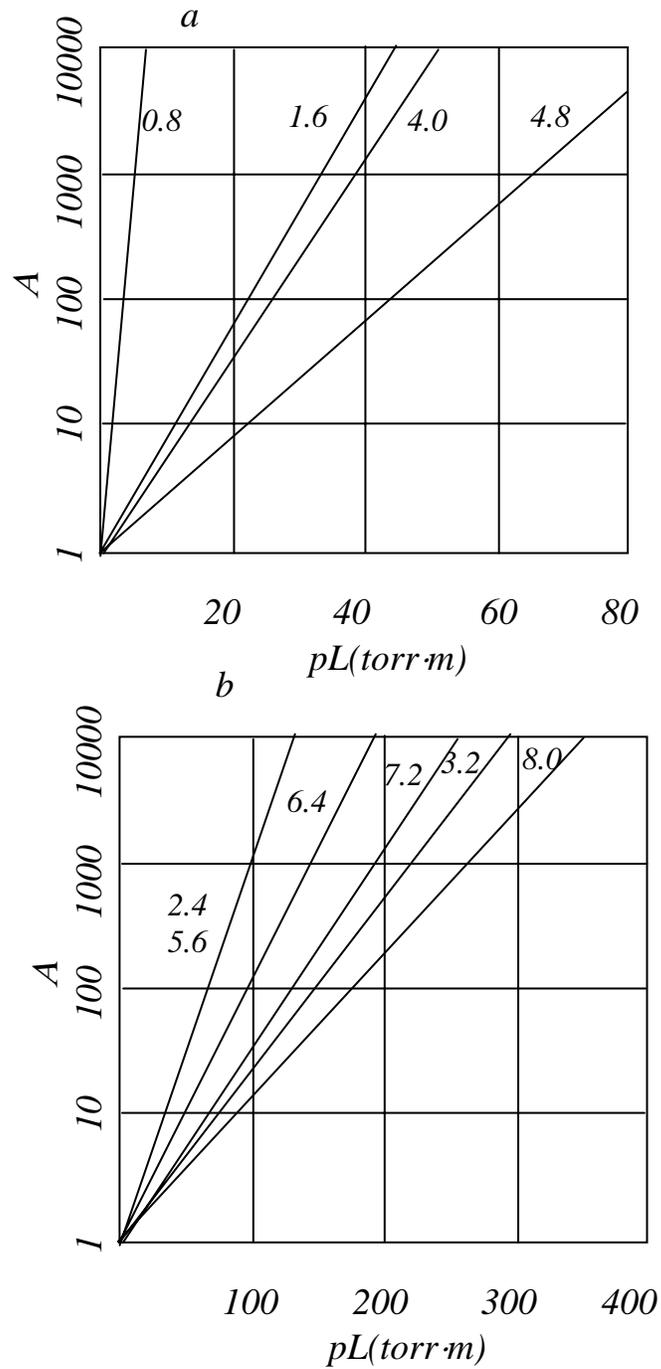
Fig.1 The dependence of the attenuation coefficient ( $A$ ) on the line-density of argon in the attenuation cell. The numbers by the lines indicate the X-ray energy in keV. We split the figure into two panels because of the difference of the horizontal scales. The lines in panel (b) for the energies 2.4 and 5.6 keV are virtually indistinguishable at this scale.
