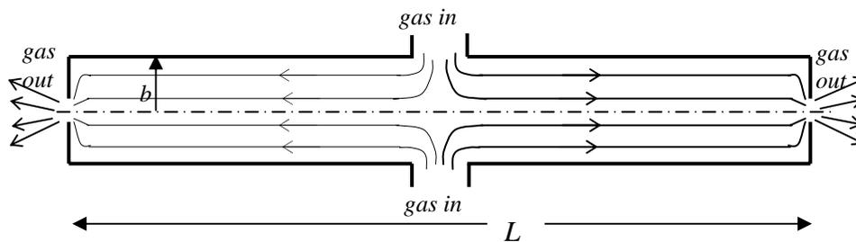
Fig. 4 Schematic of the gas flow in the attenuation cell with two gas inlets situated in the mid-plane (not to scale). The distance  $L$  is measured between the inner surfaces of the end plates. The velocity  $v$  (Eqs. (8), (9)) corresponds to the flow with straight stream-lines between the inlets and end-plates.
