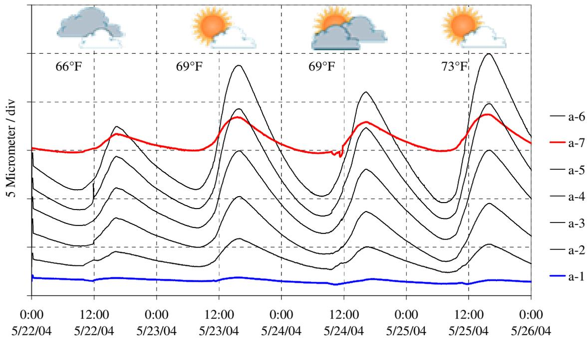
*Figure 7* Four day strip chart record of horizontal wire positions at monitors a1 to a7.
