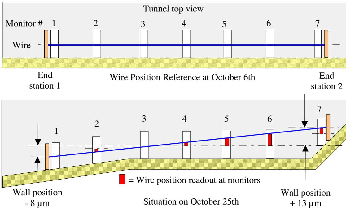
*Figure 10* Tunnel wall deforming during the October run.
