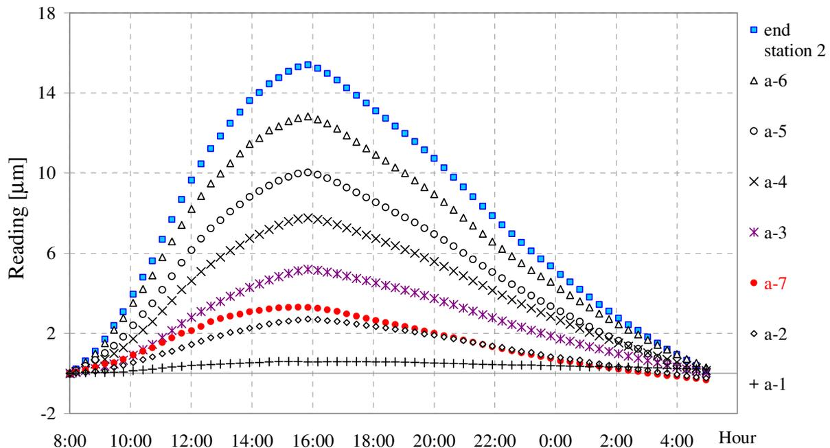
*Figure 6* Horizontal wire positions at seven monitors of wire a and position of end station 2.
