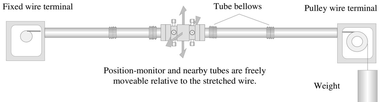
*Figure 2 Principle scheme of the stretched wire position system.*
