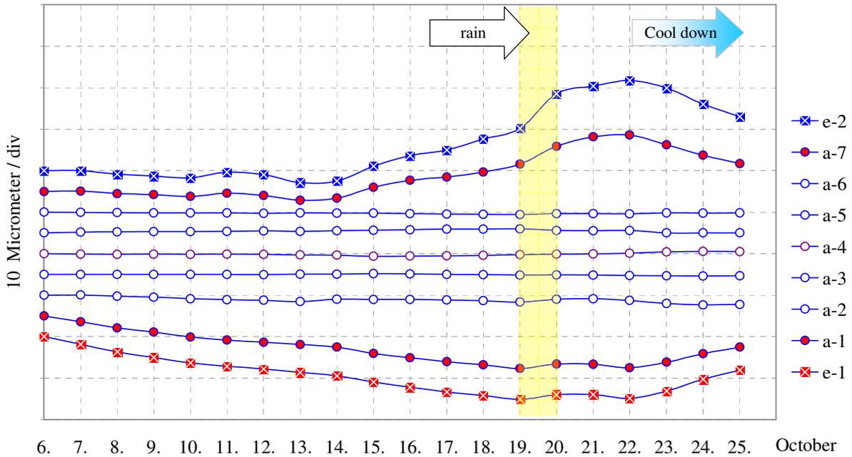
*Figure 9* Horizontal wall positions at seven monitors and two end stations. - Daily snap shots -
