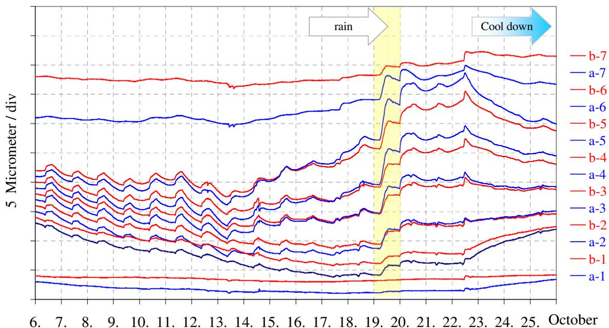
*Figure 8* Strip chart record of horizontal positions of both wires and seven monitors at each
