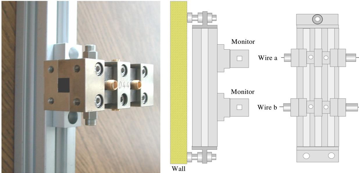
Figure 3a Wire Position Monitor front
