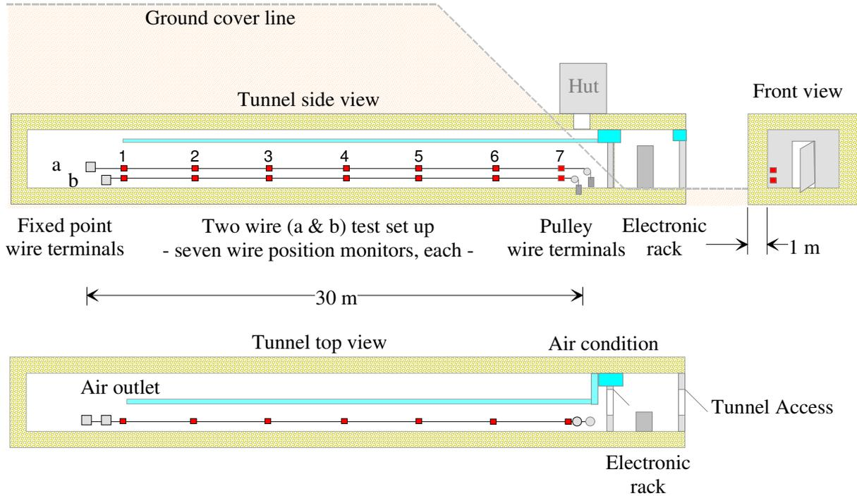
*Figure 1 Wire system test set up - geometrical layout at the Sector10 alignment tunnel -*
