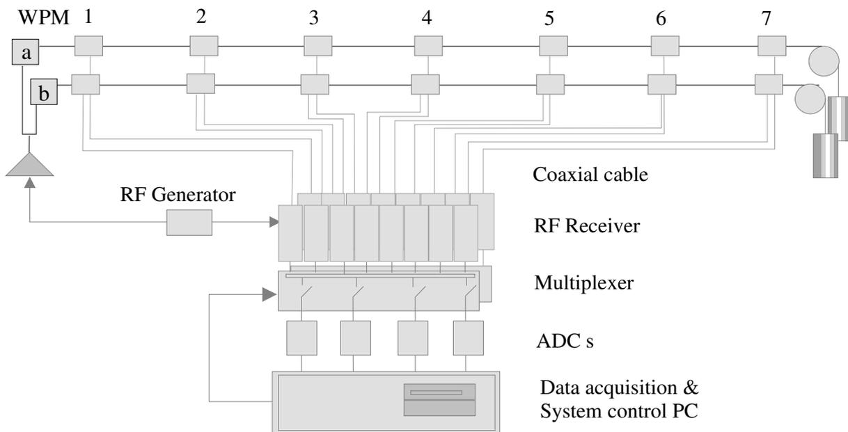
Figure 4 Wire system test set up - electrical layout and control -
