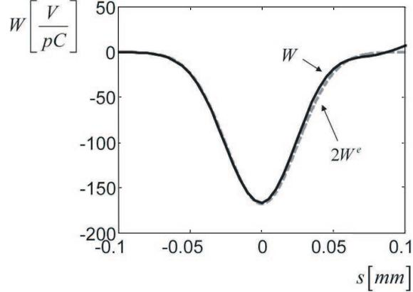
FIG. 5: Wake of a  $\sigma_z = 25 \mu\text{m}$  Gaussian bunch in the elliptical collimator (head is to the left): comparison of the indirect numerical result (solid line) with the analytical potential energy calculation (dashes).
