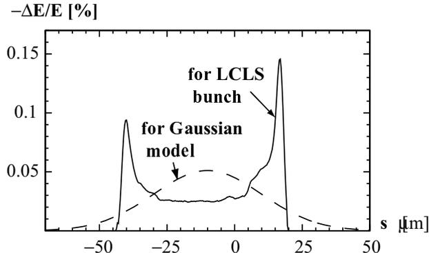
FIG. 9: Total energy change induced in the 33 pairs of rectangular-to-round transitions in the LCLS undulator region when in the 1 nC bunch charge configuration. Results are given for the actual bunch shape (solid) and for the Gaussian approximation (dashes). The head of the bunch is to the left; negative  $\Delta E/E$  indicates energy loss.
