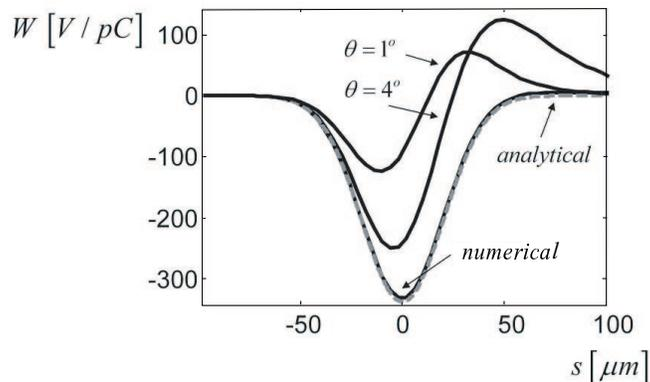
FIG. 2: Wake potential for the 2D model of a pair of LCLS transitions. The analytical result, Eq. 1, is given by dashes. Also shown are 2 results for tapered transitions (discussed below). The bunch is Gaussian with  $\sigma_z = 20$   $\mu\text{m}$  (the head is to the left).
