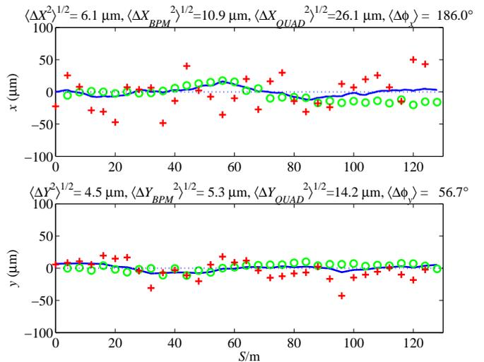
FIG. 4: Trajectories ( $x$  at top and  $y$  at bottom) after basic BBA procedure. Red crosses are quadrupole positions, blue line is electron trajectory, and green circles are BPM read-backs.
