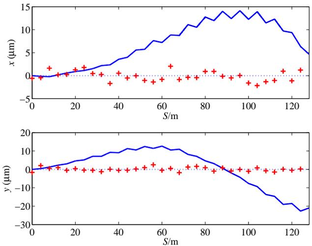
FIG. 6: Trajectories in  $x$  and  $y$  with all quadrupole magnet positions randomized by  $1 \mu\text{m}$  rms.
