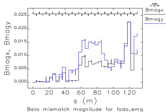
FIG. 7: Mismatch amplitude,  $\Delta\zeta$  (or "Bmag"), in  $x$  and  $y$  along undulator for random quadrupole gradients of 4% rms (Gaussian).
