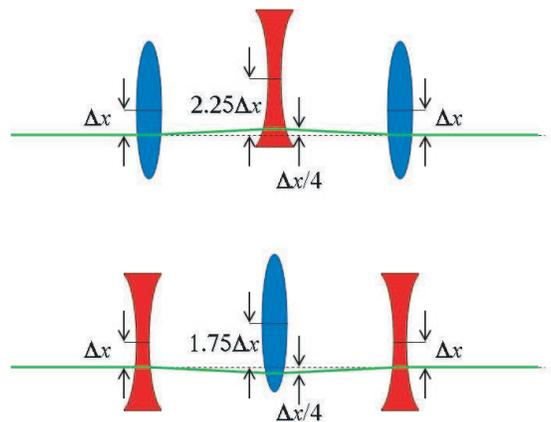
FIG. 1: Trajectory bump of three adjacent quadrupoles.
