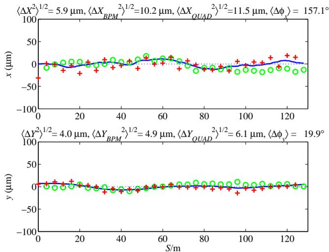
FIG. 5: Trajectory after basic BBA procedure and including local bump alignment refinement (compare to Fig. 4).
