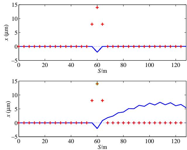
FIG. 2: Trajectory with one bump (top plot), and the same again (bottom plot) but with a relative gradient change on the central quadrupole by  $\delta = 0.2$ . Red crosses are quadrupole positions and blue line is electron trajectory.
