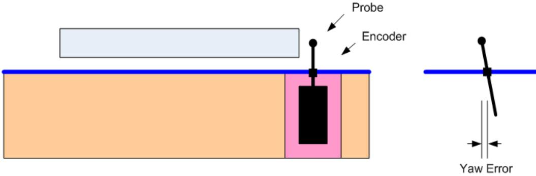
Figure 7: The measurements are triggered by an encoder on the bench. Yaw (and pitch for elevated probes) in the carriage causes the probe to be at a different  $z$  position than the trigger position.
