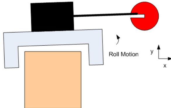
Figure 10: Roll motion of the carriage primarily causes y motion of the probe.
