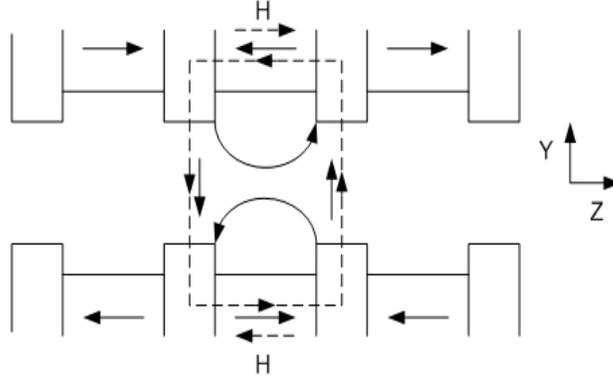
Figure 6: The dashed line shows the path used in the calculation of Ampere's law. The solid arrows show  $B$ . The two dashed arrows show  $H$  in the permanent magnet blocks.
