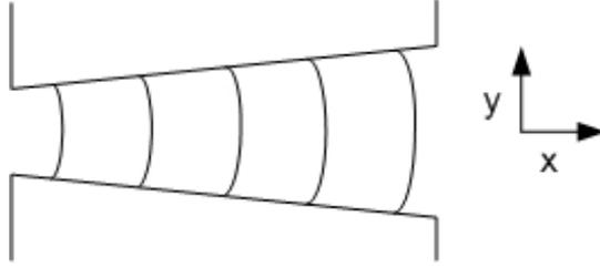
Figure 5: The poles of the undulator are not parallel. The canted poles produce a field which varies with  $x$ .
