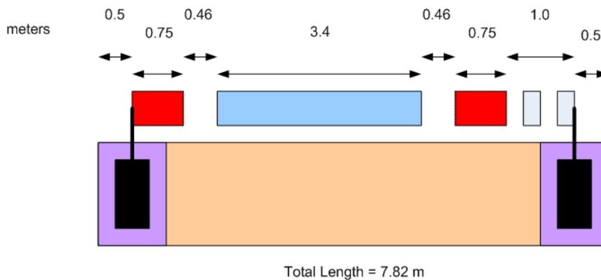
Figure 2: Measurement bench setup for stretched wire measurements.
