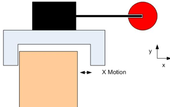
Figure 8: X motion of the carriage translates directly into x motion of the probe.
