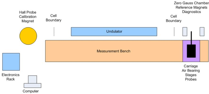
Figure 1: Overview of the LCLS undulator magnetic measurement system.
