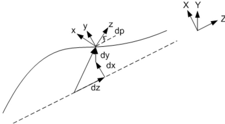
Figure 4: Probe path errors. The dashed line is the ideal probe path. The solid line is the actual path. There is a horizontal error  $dx$ , a vertical error  $dy$ , an axial error  $dz$ , and an error in the angular orientation of the probe  $dp$ .
