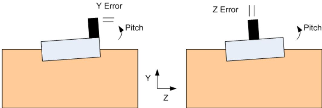
Figure 11: Pitch of the carriage causes y errors for offset probes, left, and z errors for elevated probes, right.
