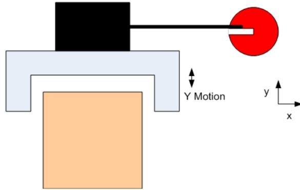
Figure 9: Y motion of the carriage translates directly into y motion of the probe.
