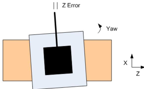
Figure 12: Yaw motion of the carriage primarily causes  $z$  motion of the probe.
