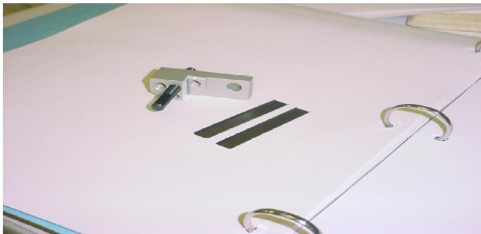
Figure 26: Pole shims and phase shims.
