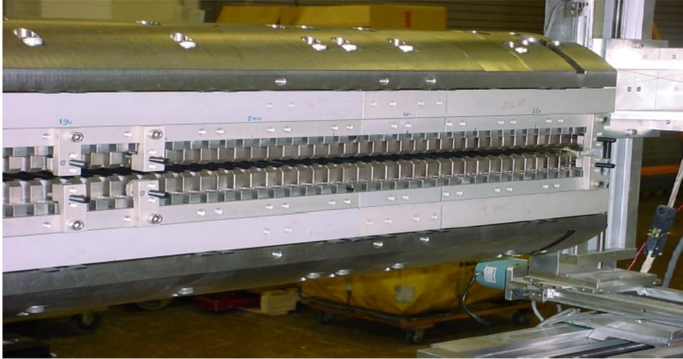
Figure 27: Shims mounted on an undulator.
