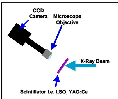
**Figure 2: Schematic of the Direct Imager X-Ray camera.**
