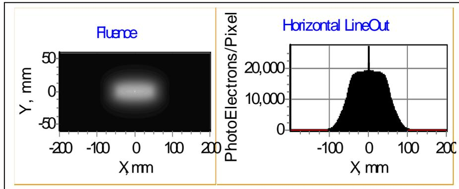
**Figure 7: Simulated Direct Imager image of the spontaneous background plus a weak ( 0.01% of saturation) FEL at 4.5 GeV.**
