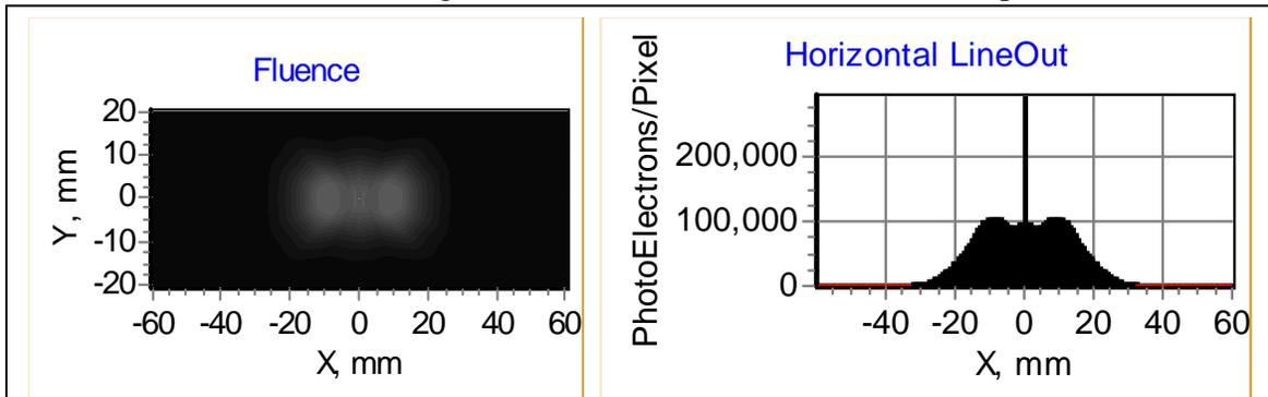
**Figure 5: Simulated Direct Imager image of a single pulse of the combined FEL and spontaneous radiation at 14.5 GeV viewed through a 16.8 mm boron carbide attenuator. The FEL was assumed to be at its full-saturated power level.**
