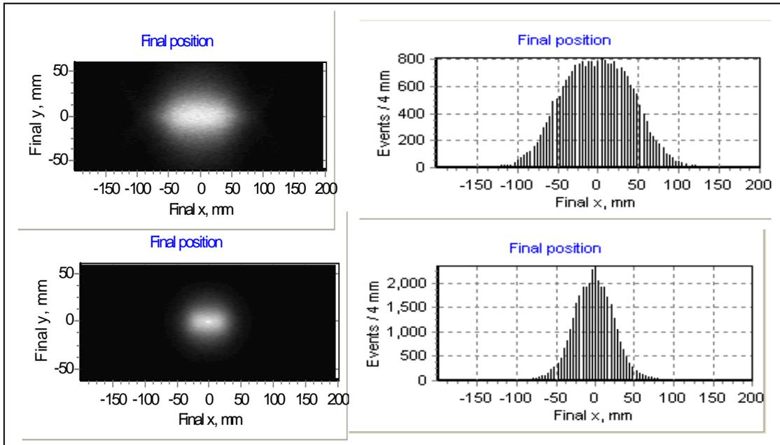
**Figure 9: Monte-Carlo simulations of the 4.5 GeV spontaneous radiation pattern at the entrance to the near hall without an undulator vacuum pipe, top, and with an undulator vacuum pipe, bottom. The spatial distribution, with the undulator pipe in place, has a FWHM of 50 mm.**
