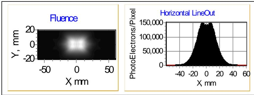
**Figure 4: Simulated Direct Imager response to a single pulse of spontaneous radiation at 14.5 GeV in photoelectrons / pixel.**
