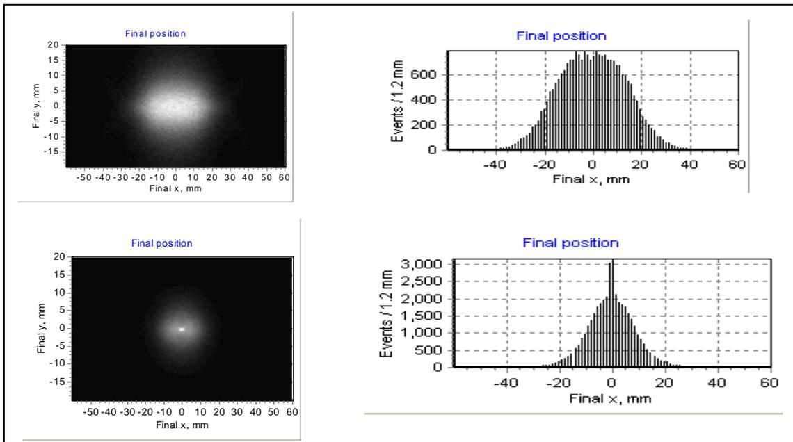
**Figure 8: Monte-Carlo simulations of the 14.5 GeV spontaneous radiation pattern at the entrance to the near hall without an undulator vacuum pipe, top, and with an undulator vacuum pipe, bottom. Almost all photons that strike the pipe reflect, resulting in a narrow, more focused spatial distribution.**
