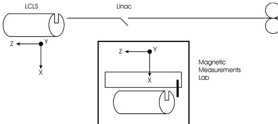
Figure 3: The undulators must be measured with the same orientation in the magnetic measurements lab as when used in the LCLS.
