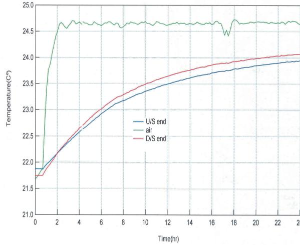
Figure 2: The undulator temperature changes at a slower rate than the air temperature. Rapid fluctuations in the air temperature do not affect the undulator temperature. This plot is courtesy of Isaac Vasserman at Argonne National Laboratory. The undulator is the first LCLS prototype.
