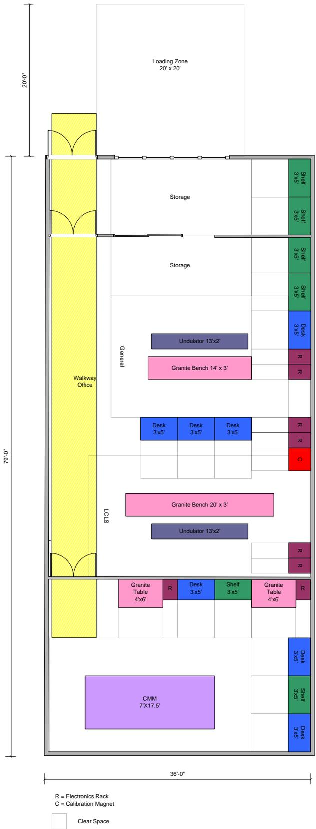
Figure 1: Possible layout of the LCLS magnetic measurement laboratory.
