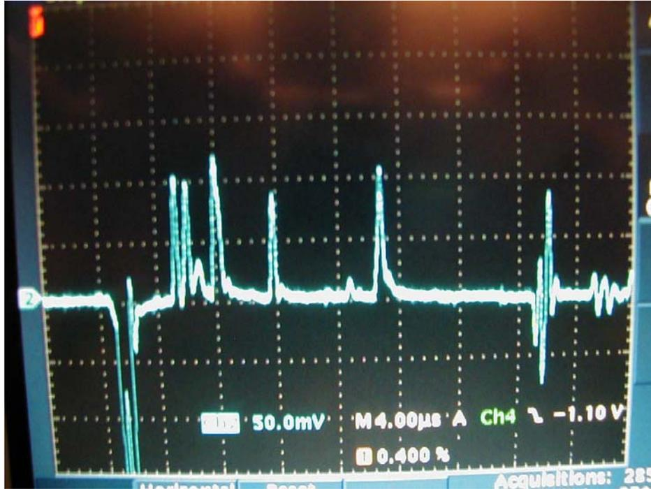
**Fig. 2.** Raw linac PLIC signal on Feb. 25, 2002, at about 09:55 for a bunch of  $5.9 \times 10^{11} e^-$ . The units are 50 mV/cm and 4  $\mu$ s/cm. Photo by Paul Miller.
