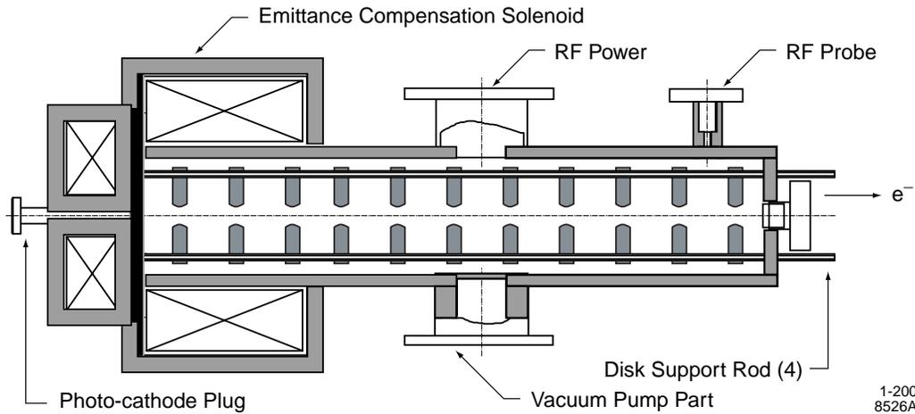
Fig. 3. Cross-section of the UCLA/Duly 1/2+10+1/2 cell plane-wave-transformer (PWT) rf gun.
