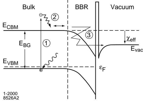
Fig. 1. Schematic energy diagram near the surface for p-doped GaAs illustrating the three-step emission process.  $E_{VBM}$ ,  $E_{CBM}$  and  $E_{vac}$  are valence band maximum, conduction band minimum, and vacuum level energies respectively.  $E_{BG}$  is the band gap,  $\epsilon_F$  the Fermi energy, and  $\chi_{eff}$  the effective electron affinity.
