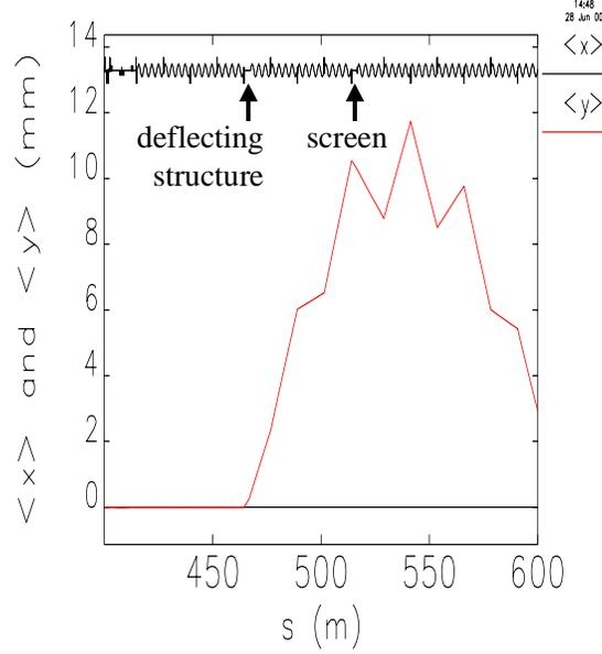
Figure 3. Vertical trajectory of beam centroid in LCLS for a 20-MV rf deflector at  $\varphi \approx 3.3^\circ$ . The second bunch compressor is located at far left in the plot. The trajectory amplitude used here is an extreme case.
