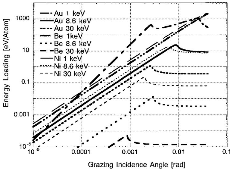
**Figure 4. Peak power energy loading of candidate LCLS mirror materials vs. (TE) grazing incidence angle**
