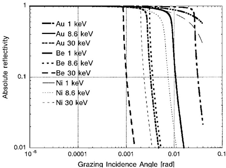
**Figure 3. Reflectivity (TE) of candidate LCLS mirror materials vs. grazing incidence angle and LCLS energy.**
