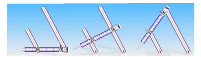
The Large Angle Detector Mover will control the position of the 2-D Detector component. Motion includes rotation about the diffractometer, tilt of the detector assemble relative to the X-Ray beamline, and X and Y position of the 2-D detector.
