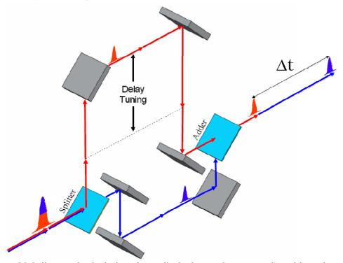
The XCS Split & Delay is designed to split the beam along two adjustable paths, recombining the two beams with an adjustable timing delay between the pulses. This device is provided with a self contained control system. Necessary vacuum components shall be integrated to the XCS Vacuum system. Ethernet access to the control system shall be provided.
