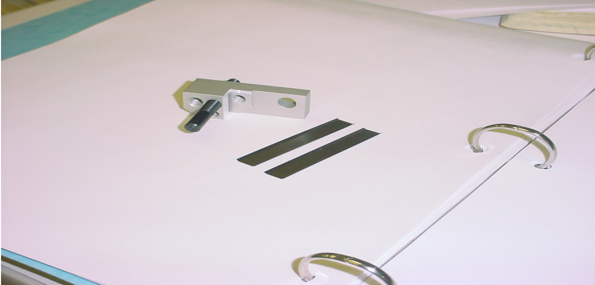
Fig. 9. Close-up view of a novel pole side shim specifically developed for small fixed-gap undulators and two regular phase shims that are placed on surfaces of the magnets. The pole side shim can use one or two threaded low-carbon steel bars (in this photograph only one bar is used).
