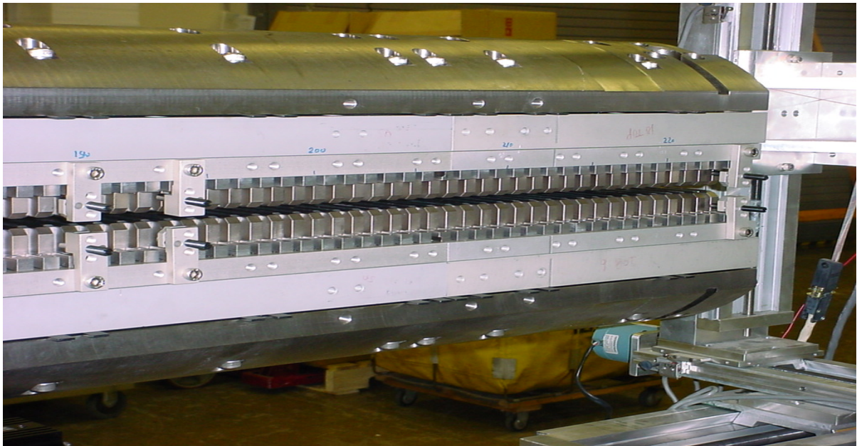
Fig. 11. Close-up photograph of the prototype undulator, which shows six pole side shims with one low-carbon threaded steel bar each, placed symmetrically at the upper and lower magnetic arrays. (Two bars per shim may be used to locally change the peak magnetic field up to about 3%.)
