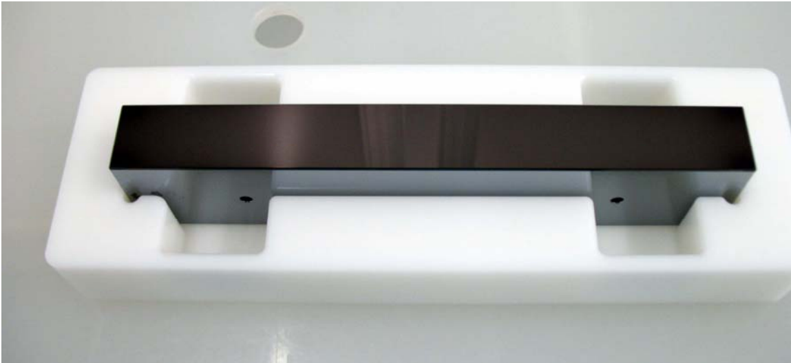
A SOMS mirror newly coated with boron carbide.
