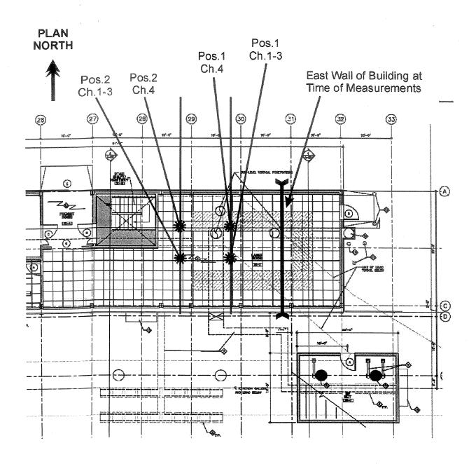
FIGURE A-1 SECTOR 20 VIBRATION MEASUREMENT POSITIONS - STREET LEVEL POSITIONS 1 & 2
