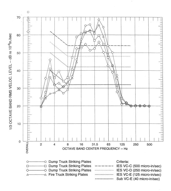
FIGURE 7D SINGLE-EVENT VIBRATION LEVELS AT POSITION 2 CH.4 - VERTICALLY PERPENDICULAR TO BEAM HALL (at 2 m) STREET LEVEL - WEST
