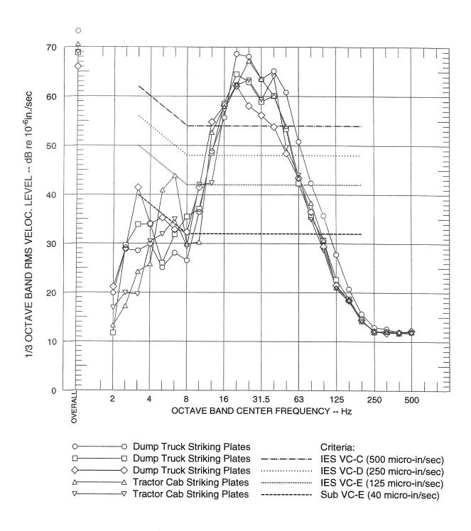
FIGURE 5D SINGLE-EVENT VIBRATION LEVELS AT POSITION 1 CH.4 - VERTICALLY PERPENDICULAR TO BEAM HALL (at 2 m) STREET LEVEL - EAST
