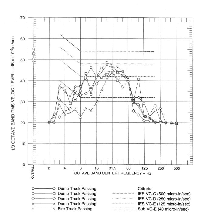
FIGURE 6D SINGLE-EVENT VIBRATION LEVELS AT POSITION 2 CH.4 - VERTICALLY PERPENDICULAR TO BEAM HALL (at 2 m) STREET LEVEL - WEST
