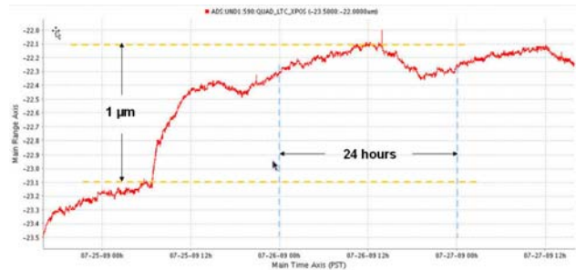
Figure 4: Horizontal position of quadrupole QU15 as monitored by the ADS over a period of about 3 days while no cam motion or segment movement occurred.
