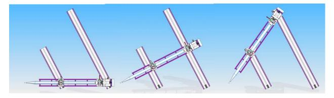
The Large Angle Detector Mover will control the position of the 2-D Detector component. Motion includes rotation about the diffractometer, tilt of the detector assemble relative to the X-Ray beamline, and X and Y position of the 2-D detector.
