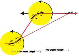
3) To achieve large offsets with single crystals, the monochromator needs to be very long. The long length impacts both cost and schedule and physically constrains the layout of experiments. The requirement for long motions might be reduced by using anti-parallel pairs in a constant offset configuration (see figure). While clearly unsuitable for a conventional synchrotron source, the extremely narrow horizontal divergence of the FEL beam might make this approach practical.
