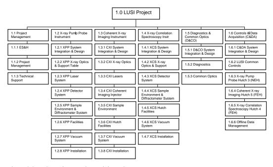
Figure 3.2 LUSI Project Work Breakdown Structure
