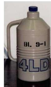
Fig. 1. Designated beam line dewar (4 liters) for filling shipping dewars.
