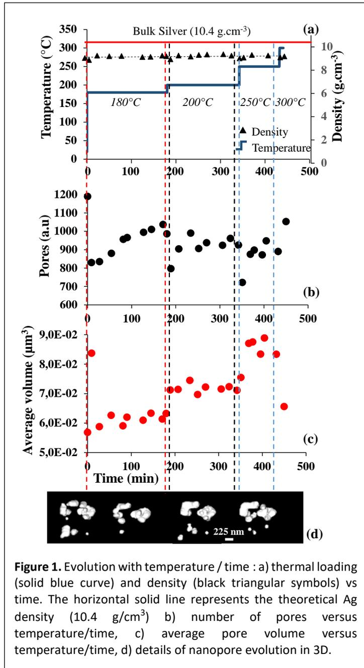
**Figure 1.** Evolution with temperature / time : a) thermal loading (solid blue curve) and density (black triangular symbols) vs time. The horizontal solid line represents the theoretical Ag density (10.4 g/cm<sup>3</sup>) b) number of pores versus temperature/time, c) average pore volume versus temperature/time, d) details of nanopore evolution in 3D.
