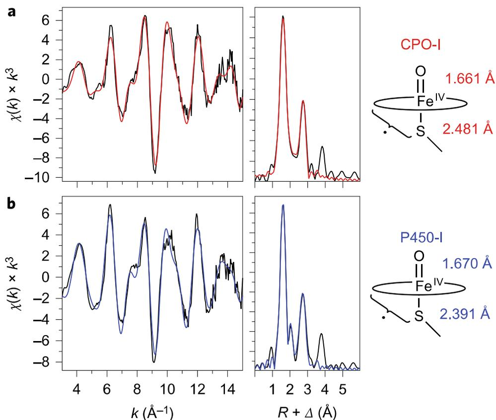
**Figure 1.** Top (a) CPO-I, bottom (b) P450-I. Left is raw EXAFS data and Fourier transforms in black and best fits in red and blue respectively. Distances on the right represent the average of multiple sets of samples for each compound. This shows a shorter Fe-S bond in P450-I as well as a slightly longer Fe=O bond compared to CPO-I.
