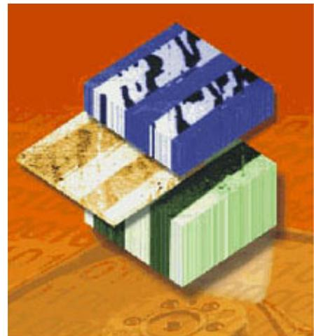
**Figure 3:** Magnetic structure, assembled layer by layer from original PEEM2 images, for a magnetic NiO (green). For the first time the magnetic structure of the interfacial CoNiO<sub>2</sub>-like layer (golden), formed by chemical reaction, could be imaged by combining chemical specificity
