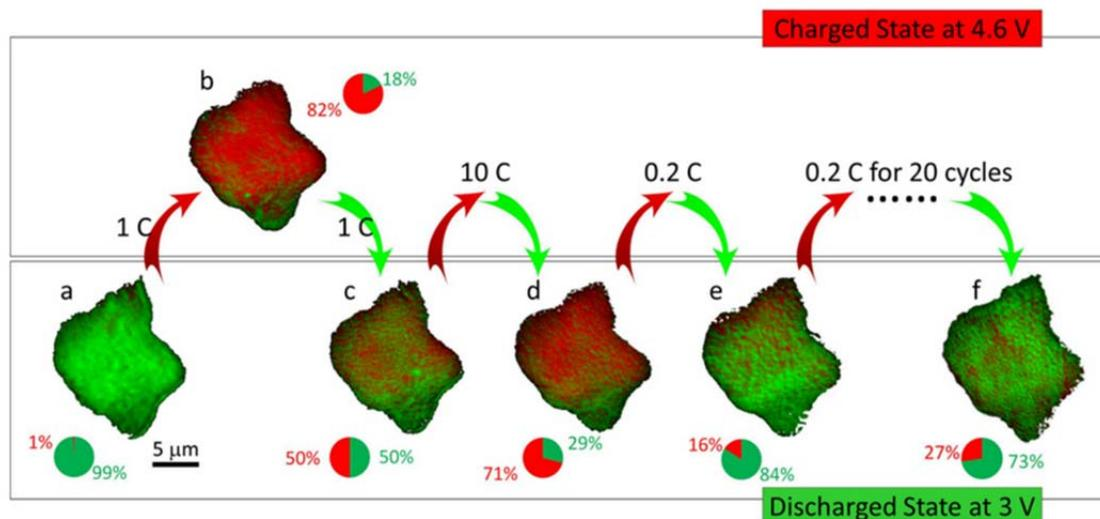
Figure 1. *In situ* monitoring of the chemical heterogeneity in a single particle of LiCoO<sub>2</sub> up to 23 cycles at different cycling rates. The red area represents the domains at charged state (Co<sup>4+</sup>), and the green area represents the domains at discharged state (Co<sup>3+</sup>).
