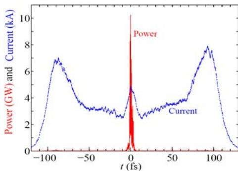
**Fig 3:** Electron current and *GENESIS* simulation of a 2 fs fwhm LCLS x-ray pulse at saturation ( $z \approx 60$  m).
