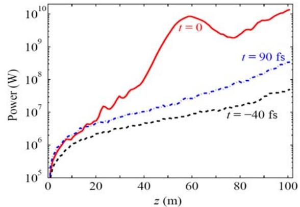
**Fig 4:** *GENESIS* simulation showing radiation power for three values of  $t$ , varying along the undulator length.
