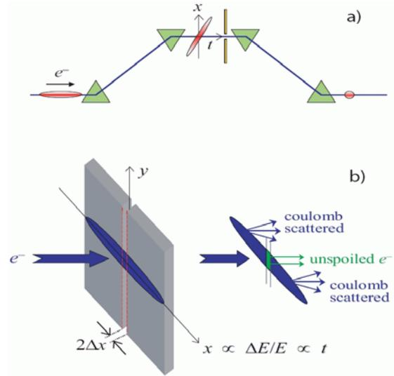
**Fig 1:** a) Sketch of an electron bunch at the center of a magnetic bunch-compressor chicane with tilted beam in horizontal,  $x$ , and longitudinal coordinates,  $t$ . b) The slotted foil at the chicane center leaves a narrow, unspoiled beam center.
