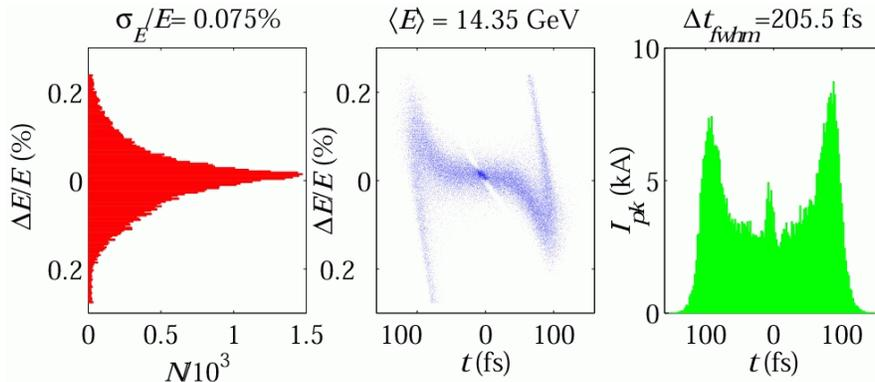
**Fig 2:** Temporal (right, peak current vs. bunch time) and energy (left, relative particle energy vs. particle count) profiles, and phase space (center) at undulator entrance. The central spike in the temporal profile is due to the slotted-foil.
