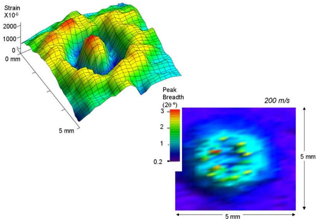
**Fig. 2.** Residual surface-normal elastic strain (upper left) and corresponding Bragg peak width (lower right) observed about a hemispherical impact crater formed at 200 m/s. For both analyses, the (21-31) diffraction peak from the dominant HCP  $\alpha$ - phase was utilized.
