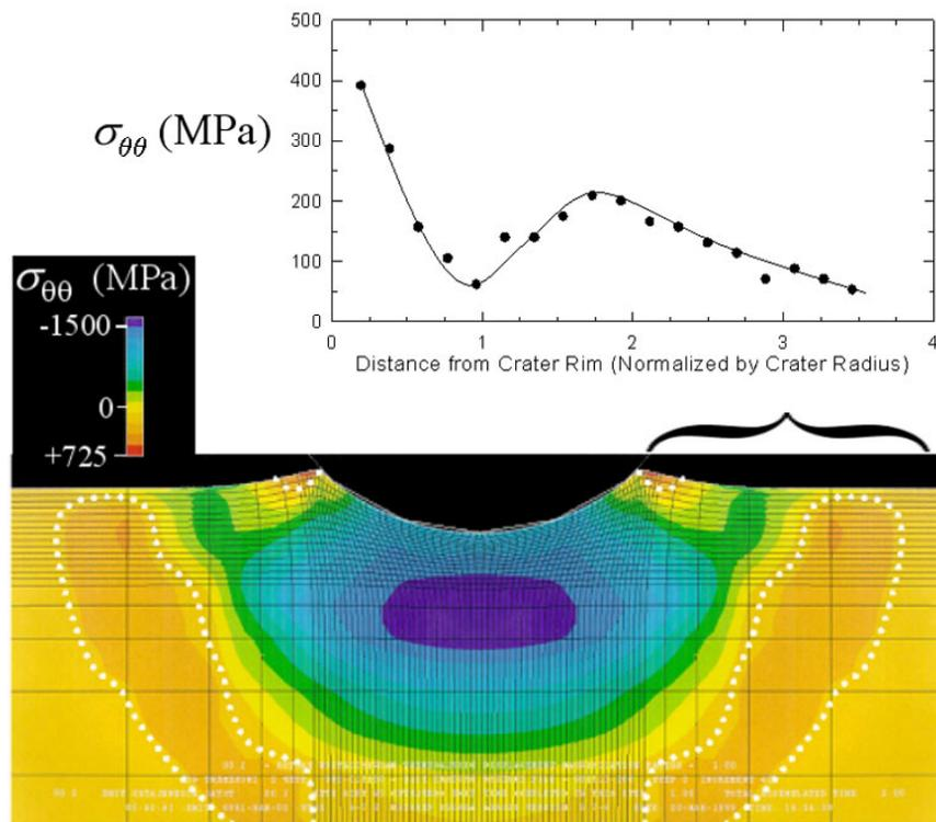
**Fig. 3.** Finite element prediction (lower contour plot) of the cross-sectional variation and experimental evaluation (upper graph) of the radial variation of residual hoop stresses for a quasi-static indent.
