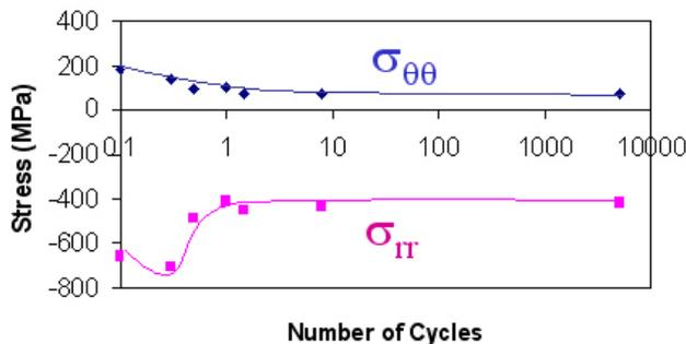
**Fig. 4.** Residual hoop and radial stress components at the crater rim, using a maximum fatigue stress of 500 MPa.
