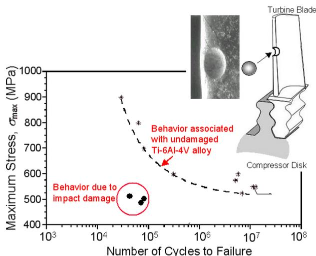
**Fig. 1.** Stress-life fatigue behavior of undamaged Ti-6Al-4V compared to impact damaged material (3.2 mm dia. spherical hardened steel projectile fired at 200-300 m/s). Load ratio,  $R = \sigma_{\min}/\sigma_{\max} = 0.1$ .
