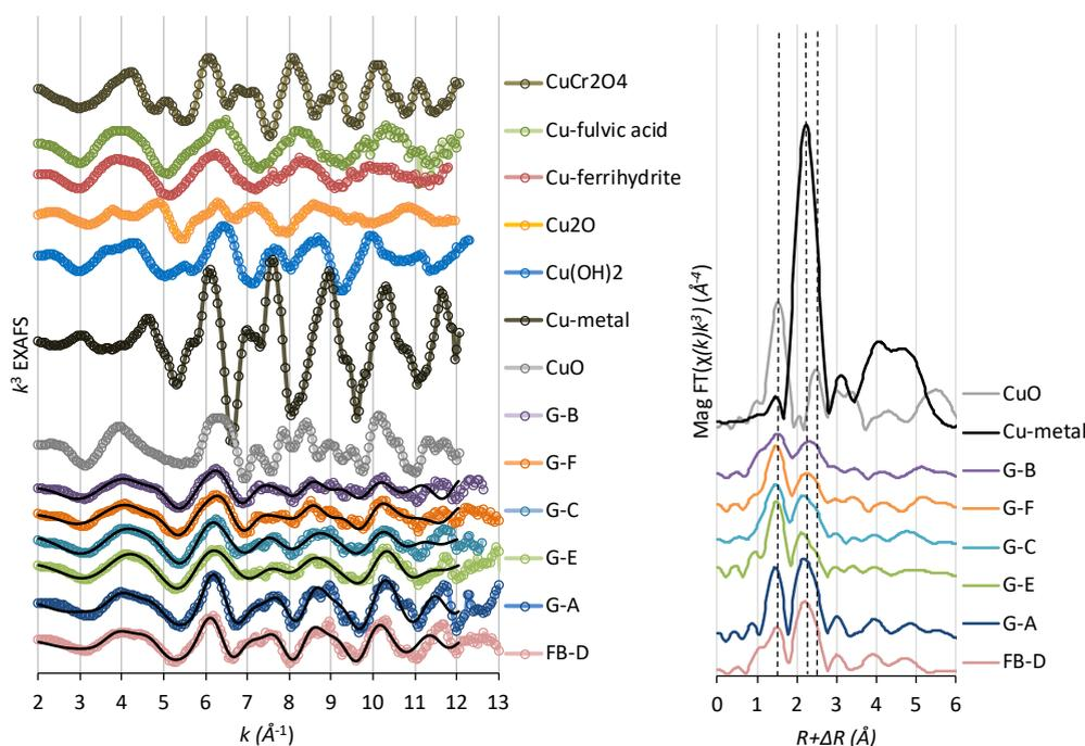
**Figure 1.** (a)  $k^3$ -weighted Cu-EXAFS spectra of standards and bottom ashes, black solid lines are fits (only ashes); (b) Fourier transforms of  $k^3$ -weighted Cu-EXAFS spectra. The first dashed vertical line marks a Cu-O distance in CuO, the second and third dashed lines mark Cu...Cu distances in Cu-metal and CuO, respectively (FT is not phase corrected).
