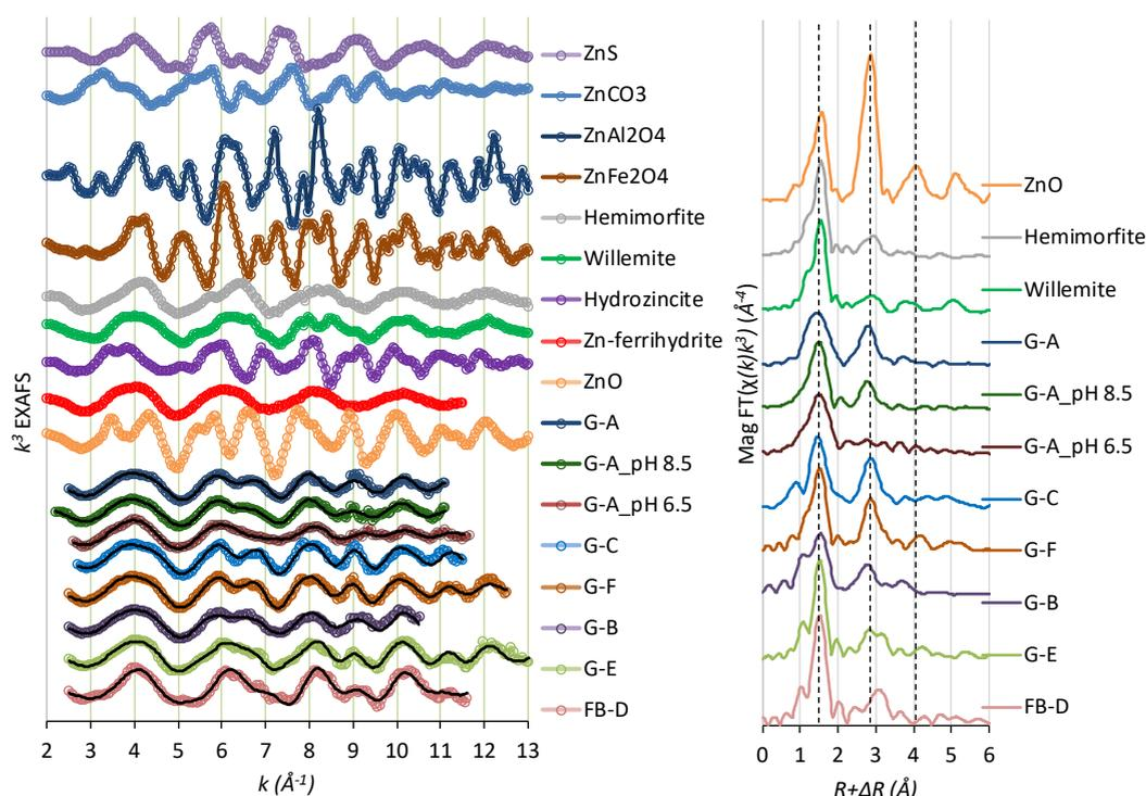
**Figure 2.** Results from EXAFS measurements: (a)  $k^3$ -weighted Zn-EXAFS spectra of standards and bottom ashes, black solid lines are fits (only ashes); (b) Fourier transforms of  $k^3$ -weighted Zn-EXAFS spectra. The first dashed vertical line marks a Zn-O distance at  $\sim 2.0$  Å. The second and third lines are Zn···Zn distances at  $\sim 3.2$  and  $\sim 4.6$  Å (the FT is not phase corrected).
